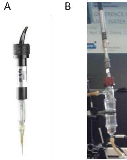
Figure 3.5. A) Nitrous oxide microsensor. B) Measurement of liquid-phase nitrous oxide in the experiments with the tubular BES.
