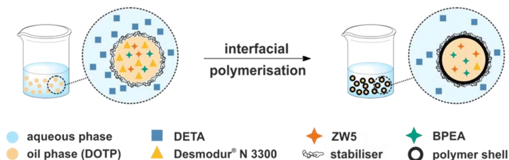
Figure 5.15 Schematic representation of the interfacial polymerisation in oil-in-water emulsions procedure used for the synthesis of polyurea capsules filled with a dye mixture in DOTP.
