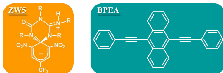
Figure 5.9 Chemical structures of ZW5 and BPEA , the dyes of choice in this chapter for the preparation of colour-tunable white-light emitting materials.
