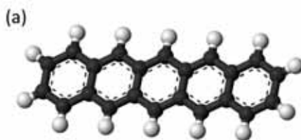
Figure 6.2.1: Molecular structure of the pentacene molecule.
