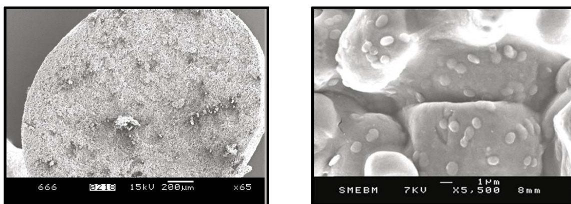
Figure 4. Scanning electron microscope pictures of alginate-starch beads: u at left, half of a biocapsule showing alginate-starch composition; at right, Raoultella terrigena immobilised on and adhered to the surface of starch granules (Schoebitz et al., 2012).
