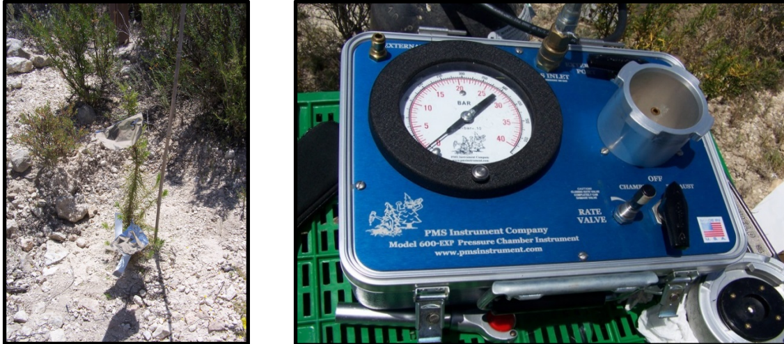
Figure 7. Stem water potential measuring by a pressure chamber.
