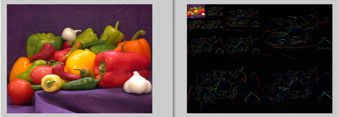
Figure 7.2: An image as example of a signal represented in traditional and wavelet basis.
