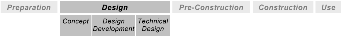
Figure 2.2. The structure of the RIBA plan of work, which indicates the stages of the design process (adapted from RIBA, 2007).
