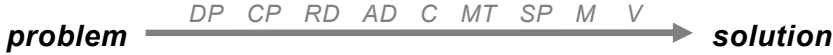
Figure 2.3. Munari represents a linear design process which leads through a sequence of phases from the design problem to the solution (figure adapted from Munari, 1983).
