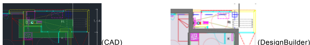
Figure 5.13. The energy assessor makes an interpretation of the design scenario when he represents it with DesignBuilder: the north wall of kitchen is simplified as a single plane in DesignBuilder.
