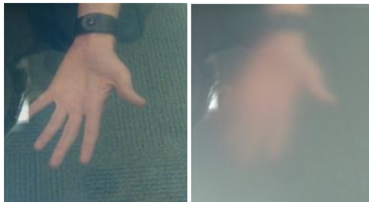
FIGURE 30: PSCT-LC STATES: CLEAR (LEFT) AND DIFFUSE (RIGHT)
