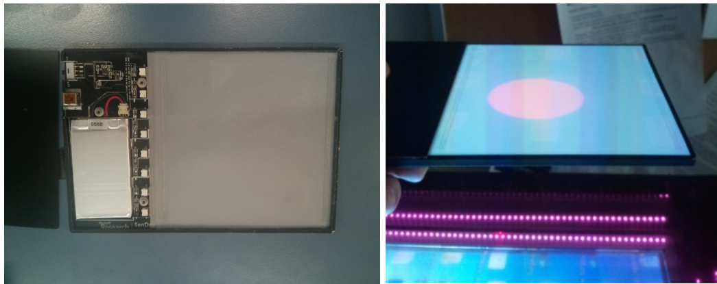
FIGURE 62: EXTERNAL DISPLAY FTIR LIGHTING (LEFT); PROJECTING A RED BALL ON AN EXTERNAL DISPLAY (RIGHT).
