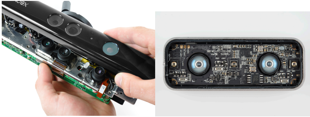
FIGURE 26: DETAILS OF A KINECT 1.0 DISSASEMBLED UNIT 35 SHOWING THE IR EMMITER, RGB CAMERA AND IR CAMERA (LEFT); DETAILS OF A LEAP MOTION DISSASEMBLED UNIT SHOWING THE TWO CAMERAS FOR STEREOSCOPIIC VISION AND THRE IR-LEDS FOR LIGHTING 36 (RIGHT)
