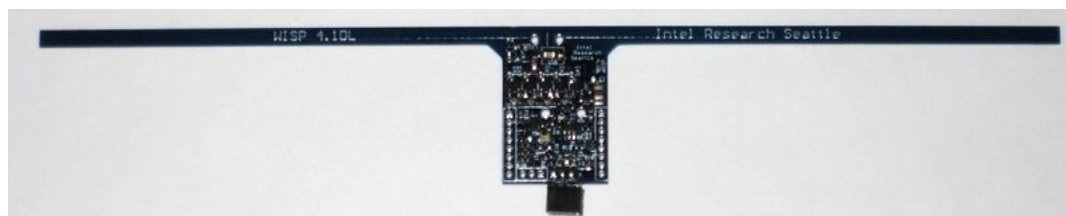
Figure 1.7. Photograph of the WISP RFID-enabled sensing platform
