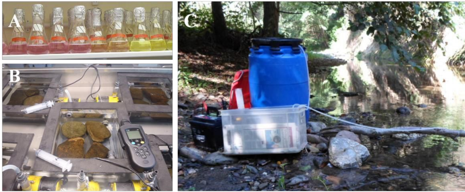
Figure 2.2: A- Stock of pure cultures of ammonia oxidizing organism used in Chapter 5; B- Recirculating chambers with oxygen probe in the water bath used in the experiments of Chapter 6; C- Experimental setting of the constant rate addition of \text{NH}_4^+ in a stream reach to measure whole-reach nitrification used in the study of chapter 7.
