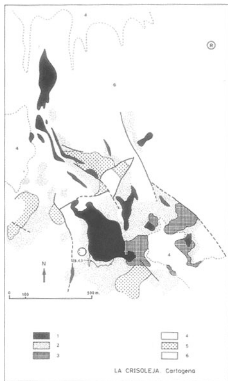
Fig. 1 “La Crisoleja” geologic simplified map. 1 Dacites with hydrothermal alteration and mineralized silica stockwork. 2 Hydrothermal alteration aureole in hosting rocks, with contact silicifications and mineralized stockwork. 3 Tabular iron silicifications. 4 Mining dumps. 5 Miocene materials. 6 Betic substrate (alpujarrides and nevado-filabrides phyllites, cherts and quartzites) (extracted and modified from Arribas et al. 1984)
