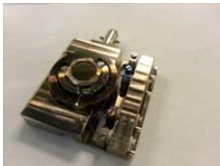
Figure 4.21: Sample mounted on the holder used for temperature experiments.
