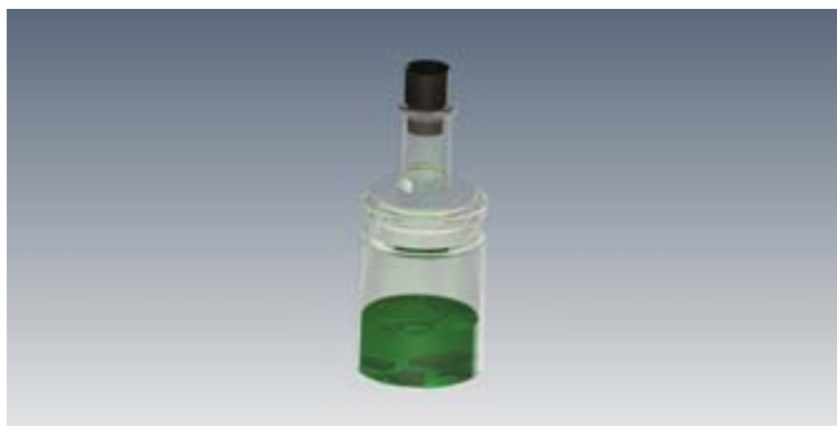
Figure 3.42: Custom-made glass container used for the fabrication of S1 and S1-H monolayers.
