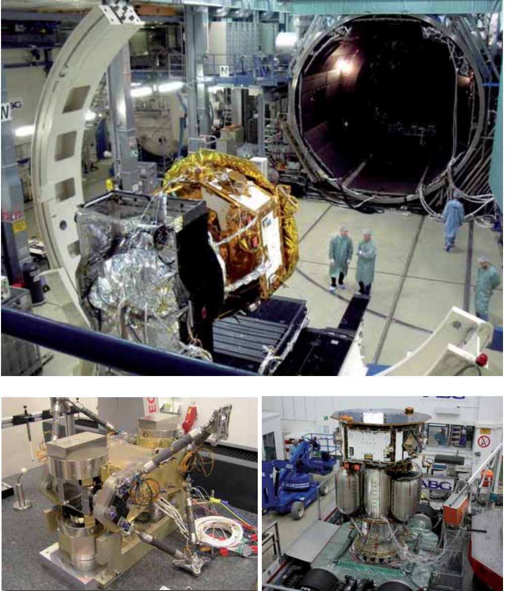
Figure 2.10: Top : IABG mbH space vacuum chamber with the LPF during the OSTT campaign. Credit: Astrium UK. Bottom left : The assembly of the TOQM thermal model. Credit: [40]. Bottom right : The LPF SC on vibration tests.
