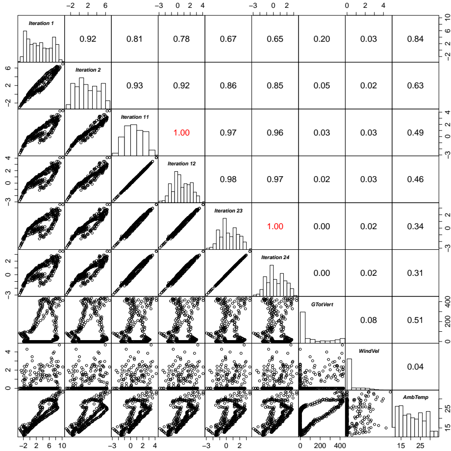
Figure 13: Correlation plots of the means of residuals among some of the iterations, Incident solar radiation ( GTotVert ), wind velocity ( WindVel ) and ambient temperature ( AmbTemp )
