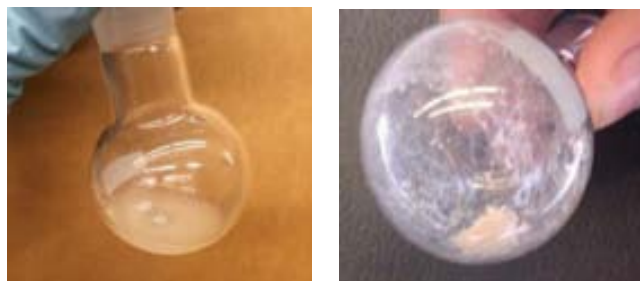
Figure 85. Appearance of the base catalyzed reaction after addition of water (left) and the resulting yellowish solid (right)
