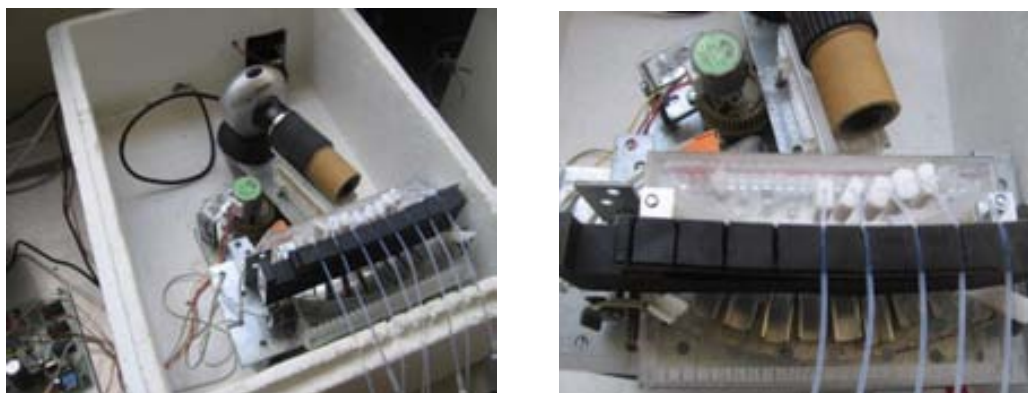
Figure 63. Surface tension measurement device designed by the Department of chemistry and technology of surfactants from CSIC (Barcelona).
