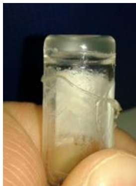
Figure 38. Tube inversion test in order to confirm the presence of the gels.
