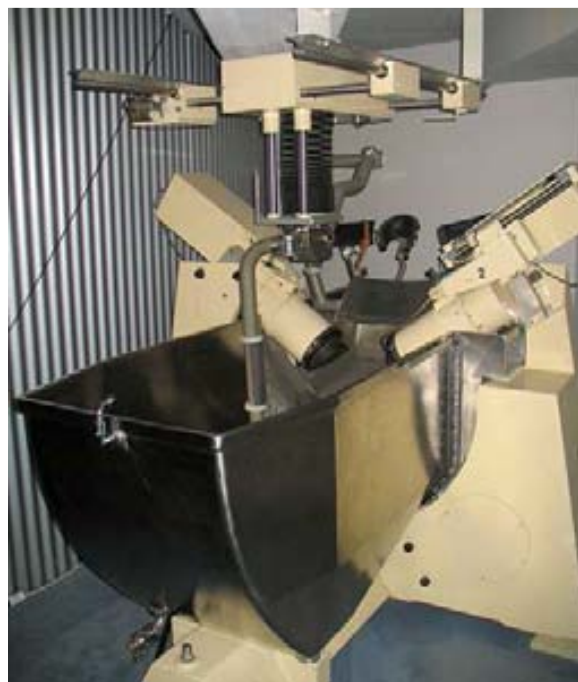
Figure 1.27 Image of the first commercially available lithotripter, Dornier MH3. Image from Dornier website 148. Of course, lithotripters have greatly evolved in terms of simplicity (they don’t use a water bath any longer) and efficacy.
