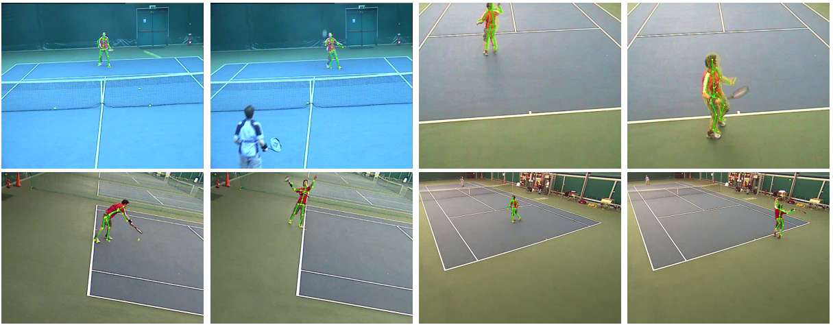
Figure 2.9: Selected frames showing pose estimates on different phases of the tennis games. The skeletal model is overlaid on the four views used for the player tracking. For clarity, we only show a wired version of the mesh body model in the second view.
