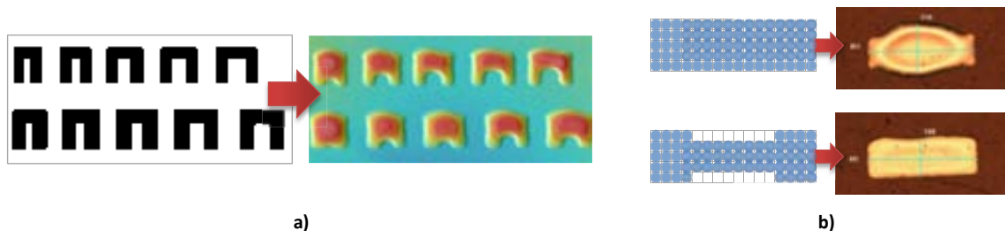
Figure 2.24. a) Deteriorated printed pattern; and b) Application of a compensation technique.
