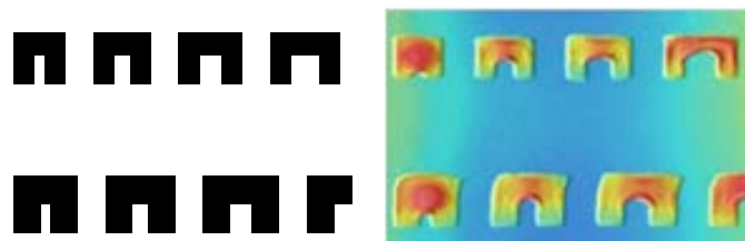
Figure 2.31. Left: Test pattern and; right: 3D image for minimum notch rule extraction.
