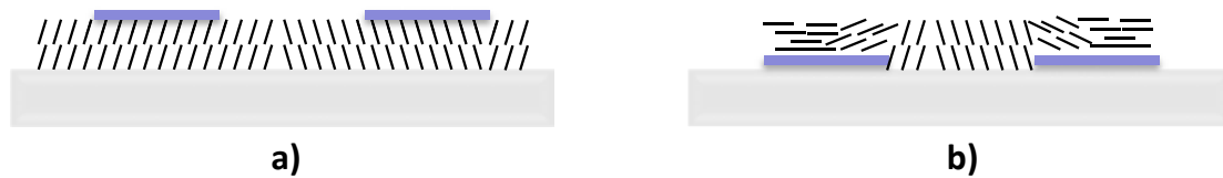
Figure 4.10. A schematic illustration of the molecular packing in: a) top and b) bottom contact OTFT devices.
