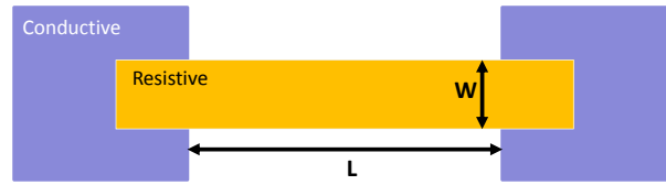
Figure 3.15. Linear resistor structure and geometry.
