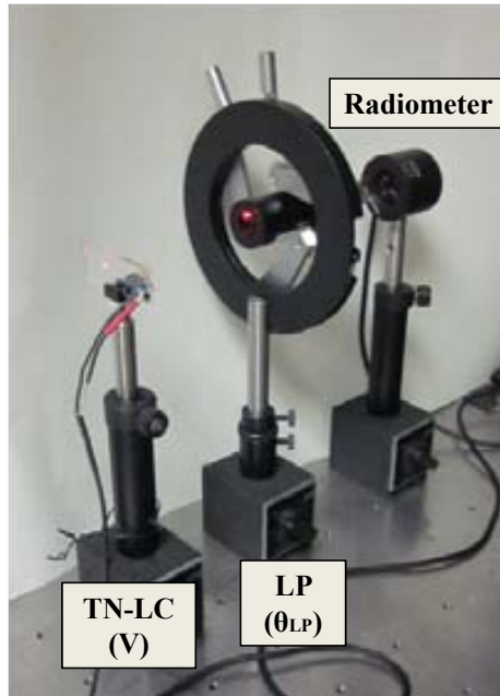
Figure 4-14: Implemented polarimeter A in our laboratory. Stokes polarimeter based on a single TN-LC panel and a linear polarizer.
