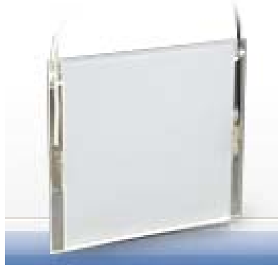
Figure 5-3: Ferroelectric liquid crystal cell used in our set-up.
