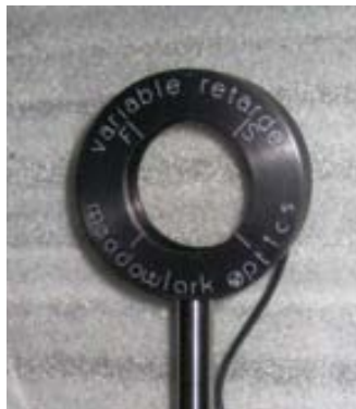
Figure 3-2: PA-LC cell used in our set-up.
