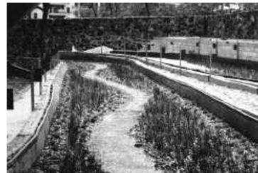
Figure 1a. River Besòs model. See the meandering low flow channel and the plastic strips on the floodplains. In the tests, the simulated vegetation completely covered the floodplains.
