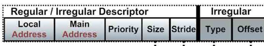
Figure 2.4: Descriptor Memory Structure: Regular and Irregular Access Patterns
