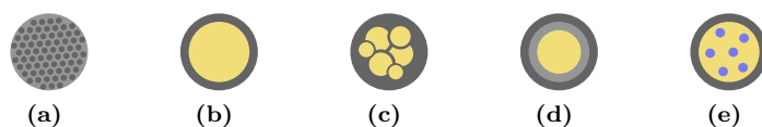
Figure 1.8: Morphology of different type of spray dried microcapsules: (a) matrix, (b) simple, (c) multi-core, (d) multi-wall, and (e) double.
