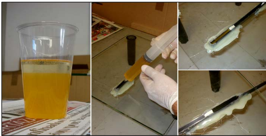
Figure 3.5. Preparation method of DLJ with low density adhesives.
