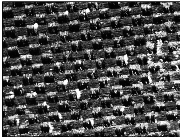
Figure 6.7. CFRP tendon failure surface of the specimen A_14_3 magnified 10x
