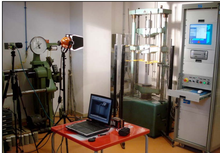
Figure 4.3. Quasi-static test setup for split-wedge anchorages.
