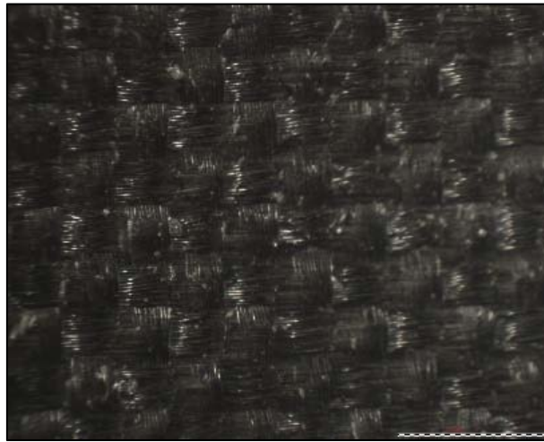
Figure 4.19. CFRP laminate failure surface of specimen DLJ_05_02_1 magnified 20x.
