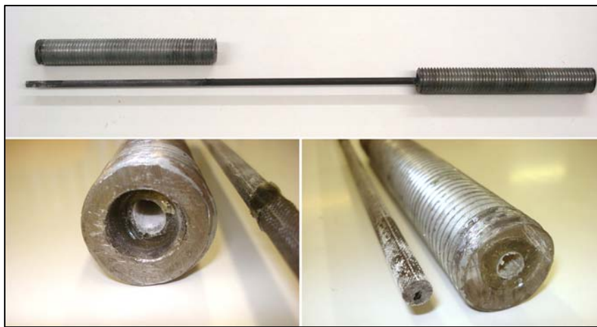
Figure 4.22. Typical failure surface in the bonded anchorages with CFRP.
