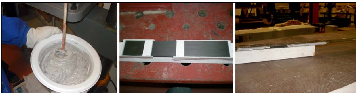
Figure 3.6. Preparation method of DLJ with high density adhesives.
