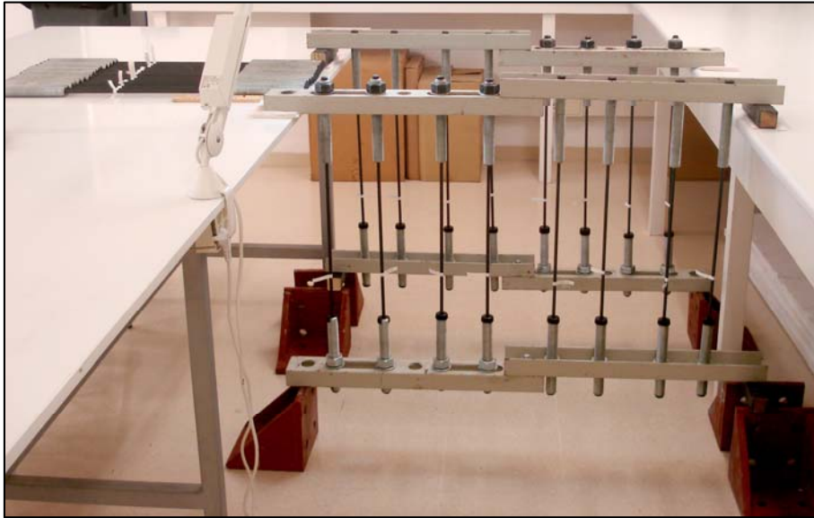
Figure 3.11. Preparation of the second anchor of straight bond-type anchorages using a double-beam.
