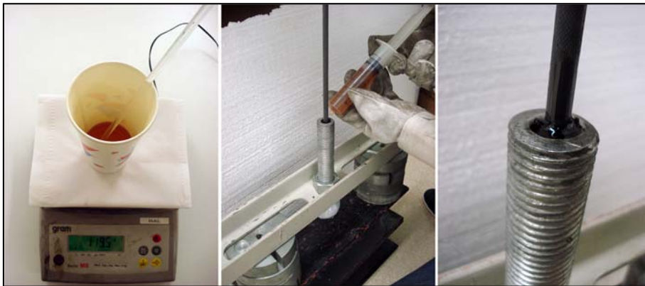
Figure 3.12. Preparation method of straight bond-type anchorage with a low density adhesive.
