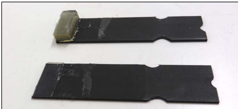
Figure 5.4. Typical failure surfaces in the SLJs.
