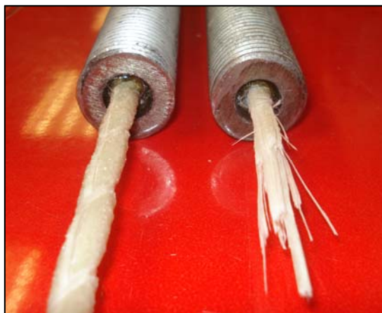
Figure 4.28. Failure mode of straight bond-type anchorages with GFRP.
