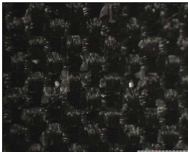
Figure 4.18. CFRP laminate failure surface of specimen DLJ_01_01_1 magnified 20x.
