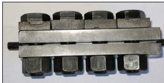
Figure 2.9. Unibody clamp anchorage for prestressing CFRP rods [15].
