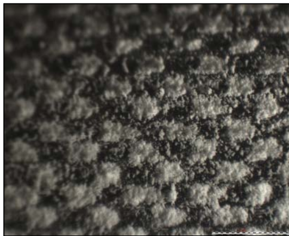
Figure 4.32. CFRP tendon failure surface of specimen A_01_02_1 magnified x20.
