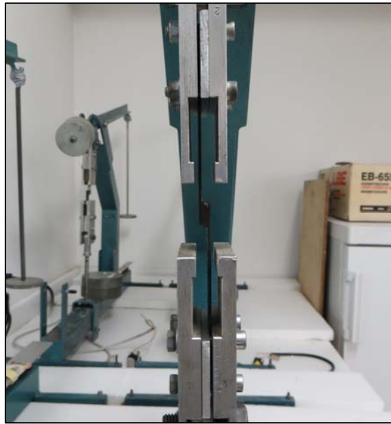
Figure 5.3. Detail of creep test setup for SLJs.
