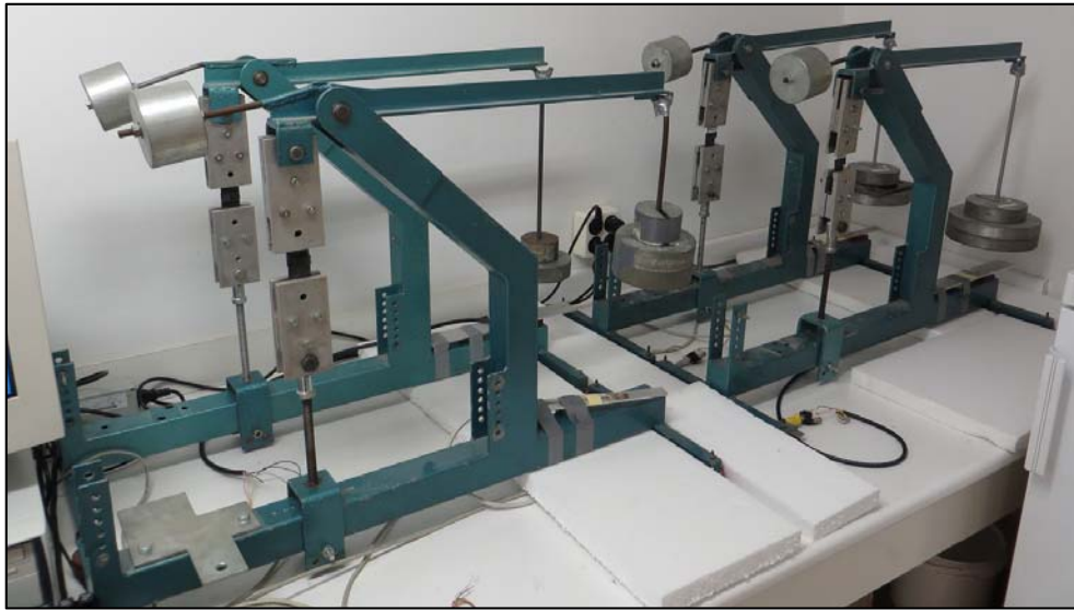
Figure 5.2. Creep test setup for SLJs.
