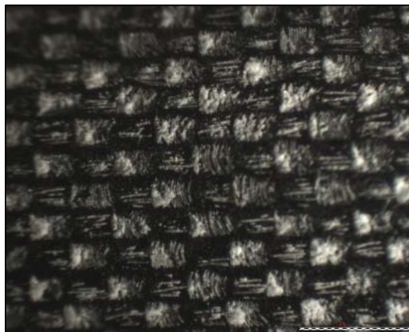
Figure 4.34. CFRP tendon failure surface of specimen A_01_02_4 magnified x20.
