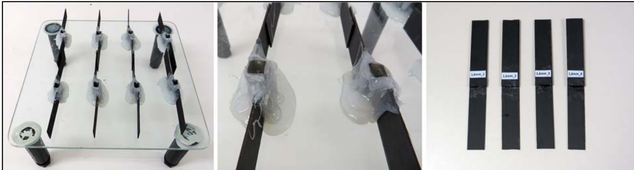
Figure 3.3. Preparation method of SLJ.
