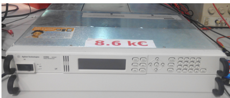
Figure A.10: PV emulator is used for making step change of irradiance or temperature E4360A.
