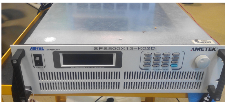
Figure A.9: Active load working as a constant voltage source SPS800X13.
