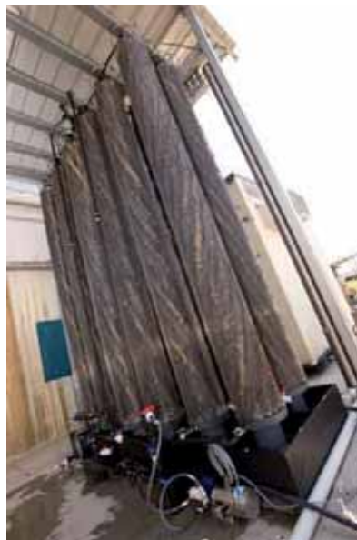
Figure 8. Pilot-scale microbial fuel cell (Image extracted from ref. 83).
