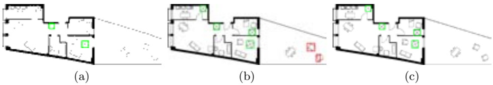
Figure 7.8: Results of spotting table1 , note that all the instances of the symbol table1 are correctly detected even the ones attached with the walls. In reality these walls are thin and hence less distorted during the vectorization, (b) Results of spotting table1 by the previous version of the method [12], (c) Results of spotting table1 by Dutta et al. [26].
