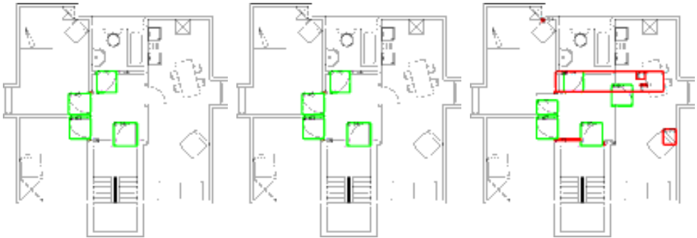
Figure 5.19: Symbol spotting: door1 . Green boxes are the true positives, the red ones are false positives.
