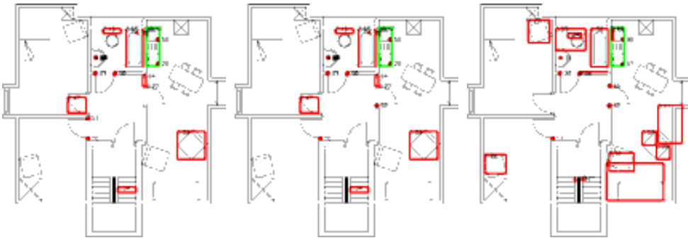
Figure 5.22: Symbol spotting: sink2 . Green boxes are the true positives, the red ones are false positives.
