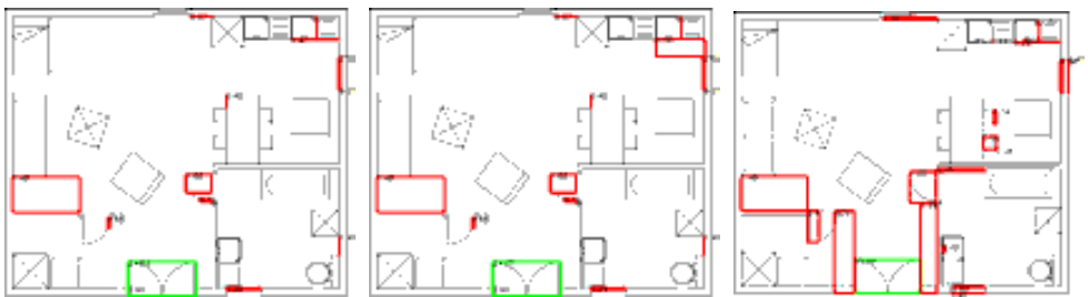
Figure 5.20: Symbol spotting: door2 . Green boxes are the true positives, the red ones are false positives.
