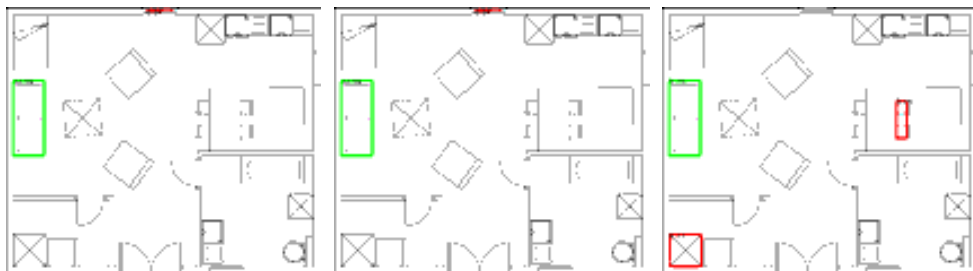
Figure 5.24: Symbol spotting: sofa2 . Green boxes are the true positives, the red ones are false positives.
