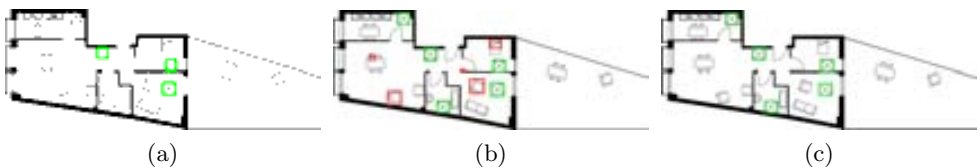
Figure 7.10: Results of spotting table1 , note that all the instances of the symbol table1 are correctly detected even the one which is connected with thick black pixels, (b) Results of spotting table1 by the previous version of the method [12], (c) Results of spotting table1 by Dutta et al. [26].
