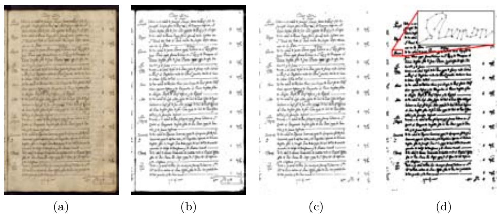
Figure 4.16: An image from the marriage register from the fifth century from the Barcelona cathedral, (a) The original image, (b) The binarized image of 4.16a, (c) The image in 4.16b after preprocessing (eliminating black border created due to scanning), (d) Graph constructed from the image in 4.16c: the inset also shows the zoomed part of a word Ramon .
