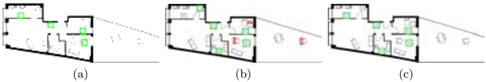
Figure 7.9: Results of spotting table1 , except one all the instances of the symbol table1 are correctly detected. The one which is not detected is attached with the thick black pixels, (b) Results of spotting table1 by the previous version of the method [12], (c) Results of spotting table1 by Dutta et al. [26].
