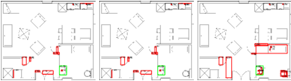
Figure 5.21: Symbol spotting: sink1 . Green boxes are the true positives, the red ones are false positives.
