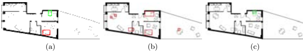
Figure 7.6: Results of spotting bed , here the single instance of bed is correctly detected, note that in this case the instance is also attached with thin black pixel, (b) Results of spotting bed by the previous version of the method [12], (c) Results of spotting bed by Dutta et al. [26].
