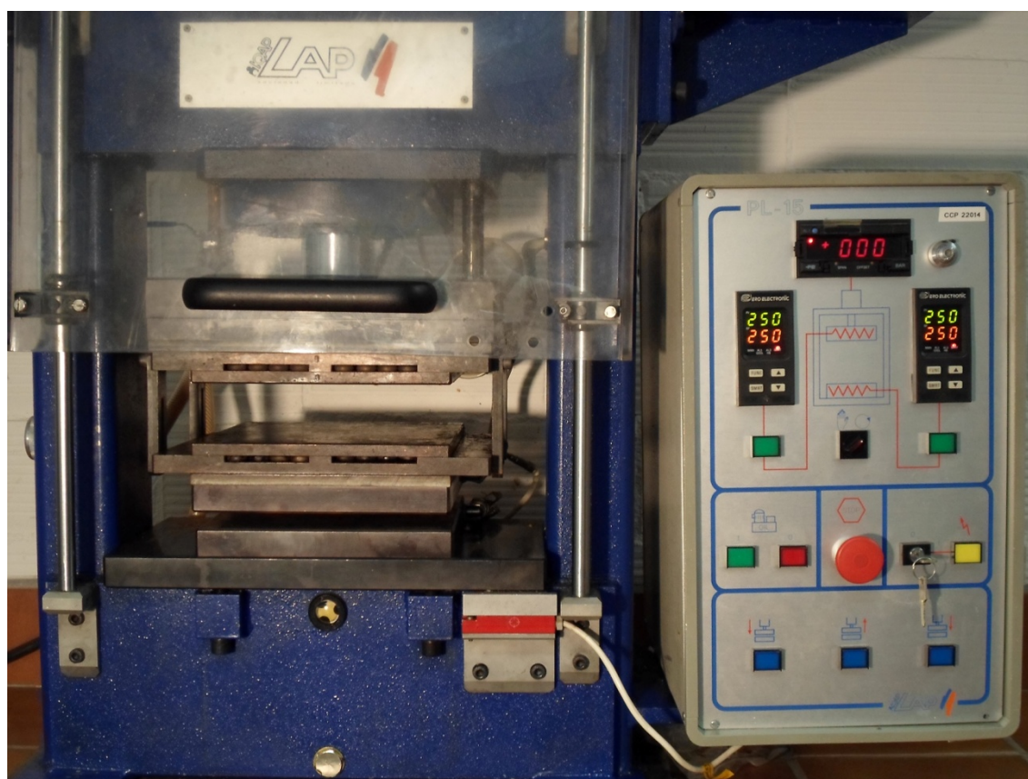
Fig. 4.1: IQAP LAP PL-15 hot plate press equipped with temperature- and pressure-controlled plates
