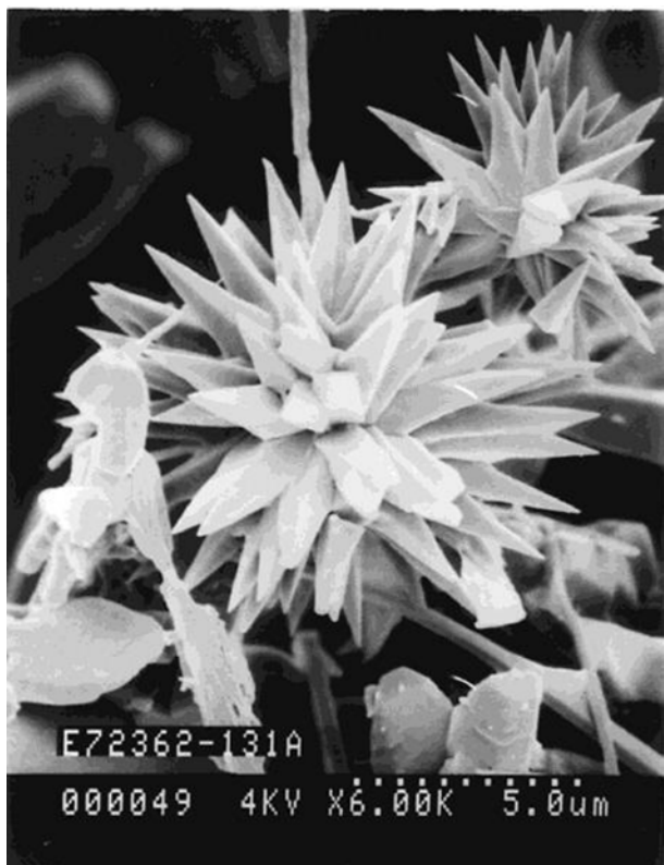
Fig. 2.15: Scanning electron microscopy showing the particle morphology of cyclic PET oligomer crystals produced by solvent-induced crystallization in hexadecane, adapted from [32].
