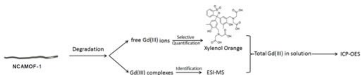
Figure 21. Analytical strategy to evaluate NCAMOF-1 degradation in water and physiologically simulated conditions.
