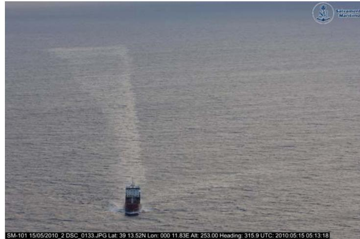
**Figure I-17** Oil slick trail from a polluting vessel detected using airborne visible optical sensor (EMSA, 2010).
