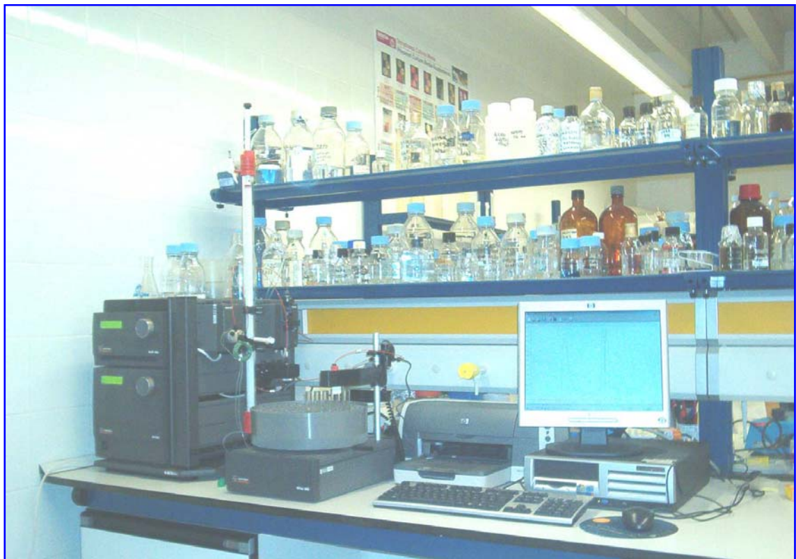
Figure M.1 AKTA FPLC (Fast Protein Liquid Chromatograph).
