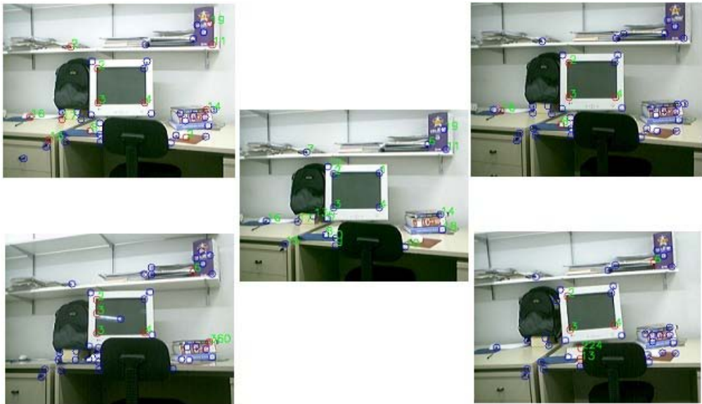
Figure 5.4 Descriptors created in the learning phase (central image). Examples of descriptors matched in the recognition phase: (upper-left image) case a : little change in 3D point of view and little change in illumination; (upper-right image) case b : Little change in 3D point of view and medium change in illumination; (lower-left image) case c : a change of 20 degrees in the 3D point of view and medium change in illumination; (lower-right image) case d : a change of 10 degrees in 3D point of view, 5 degrees in rotation and medium change in illumination.
