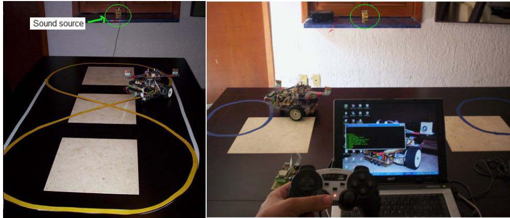
Figure 4.23 Experimental Setup: Robot tracking a predefined path using its line-tracking sensor (left). Robot manually driven by a joystick (right). Note the Sound Source at the middle-upper of the pictures.
