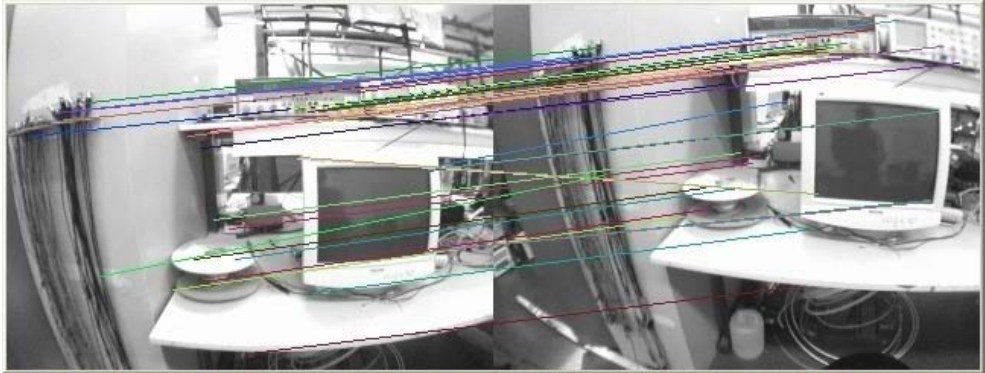
Figure 5.7 Two images were taken with different point of view of some area in a laboratory. 46 matches were found using SIFT descriptors, 6 been false positives. In general SIFT descriptors gives impressive results; however in Kalman-based SLAM a few mismatches can be enough for producing divergence in the filter.
