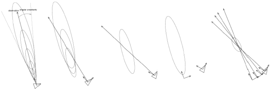
Figure 4.4 Sola and Lemaire feature initialization. From left to right: the sum of Gaussians is initialized in the robot frame; some Gaussians are pruned based on their likelihood after additional observations of the feature; when a single hypotheses remains, the feature is projected into the map frame; and finally past observations are used to update the feature estimate. (Graphics taken from [114] ).
