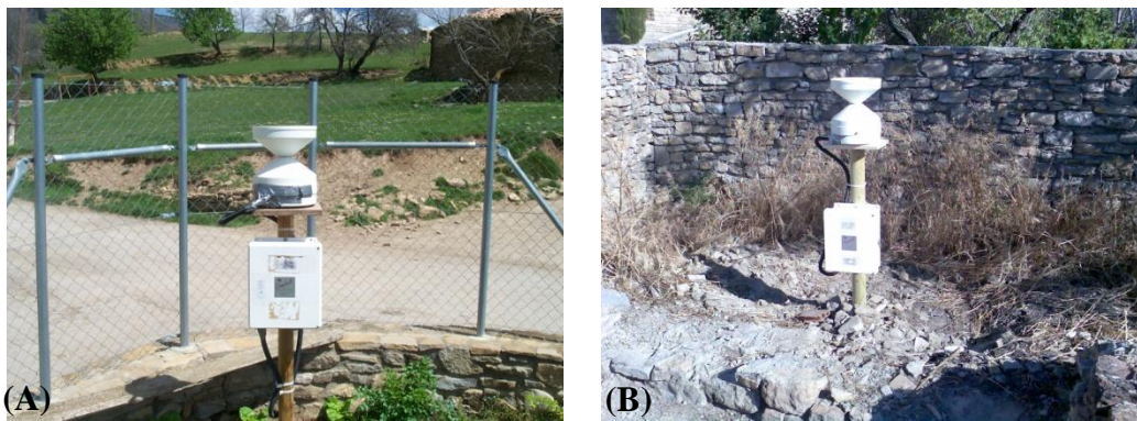
Figure 2.8. Campbell ARG100 tipping-bucket rain gauges installed at (A) Villacarli and (B) Roda de Isábena.
