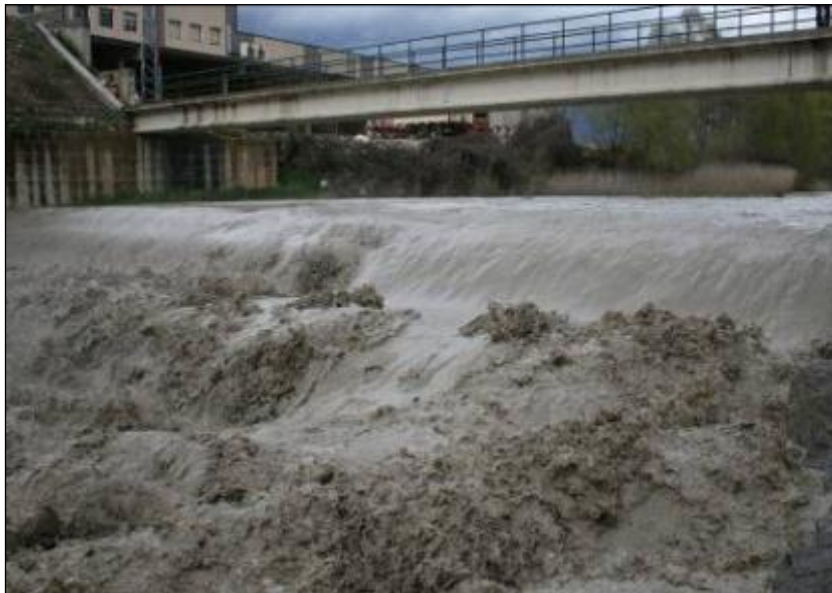
Figure 1.2. High density flow observed at the Capella gauging station (outlet of the Isábena basin) during a flood in April 2008.
