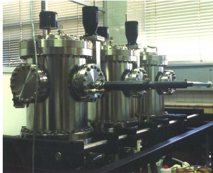
Fig. 2.1. Picture of the multichamber HWCVD set-up. The system was fabricated by the Scientific-Technical Services of Universitat de Barcelona.
