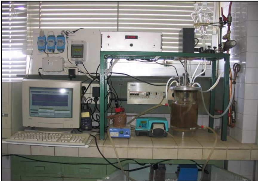
Figure 3.5 – Closed Intermittent-Flow respirometer constructed in this study. Scheme of the respirometer (a) and photograph of the experimental device (b).
