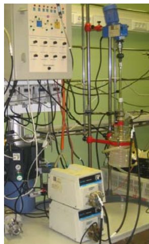
Figure 3.4 – Anammox SBR of 1L tested in this work.
