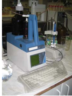
Figure 3.14 – Titrator used to perform alkalinity measurements.
