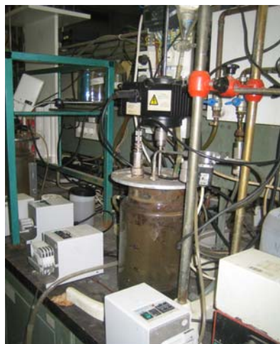
Figure 3.3 – Lab-scale SHARON reactor (4L) used in this study.
