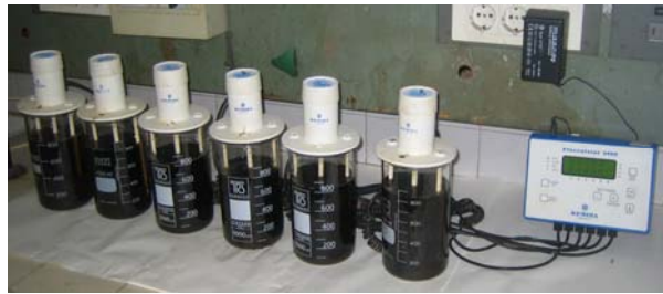
Figure 3.9 – Jar-test device used in this study.
