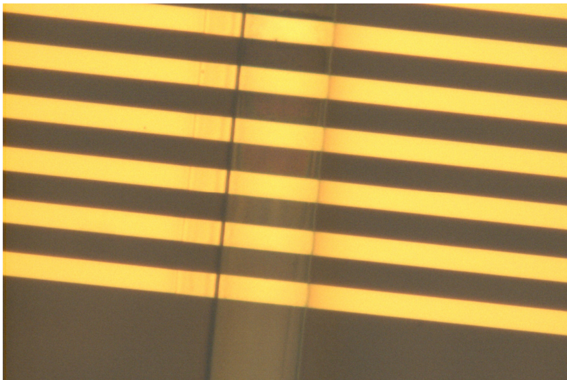
Fig. 2 Optical image of the microfluidic channel crossing the set of gold microband electrodes. The working area of the electrodes is determined by the width of the gold bands ( 14\text{ }\mu\text{m} ) and the width of the channel ( 50\text{ }\mu\text{m} ).
