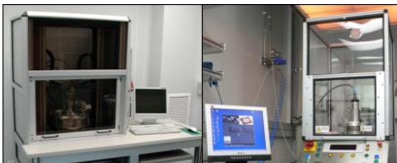
Fig. 4 Pictures of the Hot Embossing system (HEX01, Jenoptik AG, Germany) (left) and Nanoimprint Lithography system (Obducat, Sweden) (right) used to imprint and bond, respectively, the pillar array structures.
