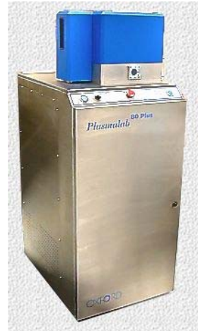
Figure 2-41 a) Draw of the RIE machine. A gas is inserted in the chamber and an RF field produces plasma (pink), the plasma attach the sample. b) Picture of the Plasmalab 80 from Oxford Instruments used at Parc Científic de Barcelona.
