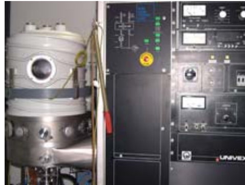
Figure 2-39 a) Schematic draw of the vacuum chamber of a Evaporator machine. b) Picture of the Univex 450 by Leybold.
