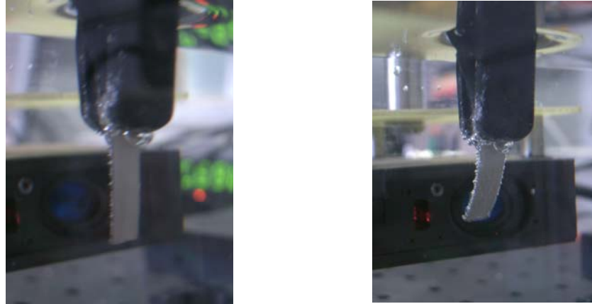
Figure 2-20 Bubbles formed in water due to hydrolysis when driving IPMC with 5V. a) straight beam, b) bend beam.
