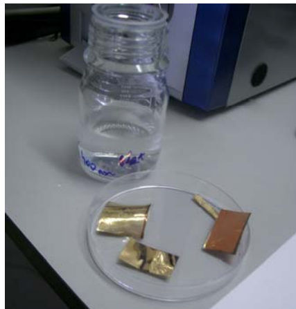
Figure 2-43 Picture of the samples, the golden are not treated with RIE and the mate is treated with RIE.
