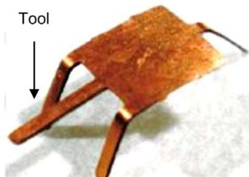
Figure 2-11 Picture of the locomotion and sensor platform of the ISWARM microrobot. Picture obtained from Snis_2008_2.
