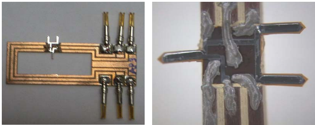
Figure 2-6 a) Picture of the PCB with the electrical connector pins. b) Zoom of the legs with the conductive glue.
