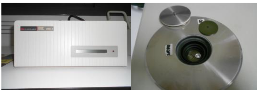
Photo 12: DSC, Differential Scanning Calorimeter
