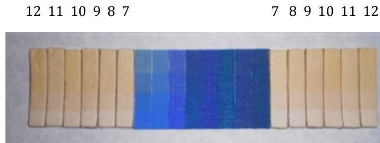
Photo 4: Light Fastness for experimental part 4.2, (samples 7-12)
