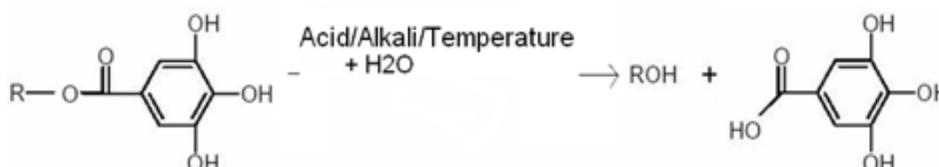
Figure 17: Formation of free Gallic acid by hydrolysis of hydrolysable tannin
