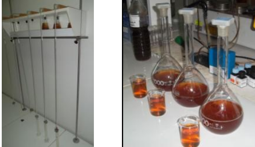
Photo 5: Photographs of the tannin determination method assembly.
