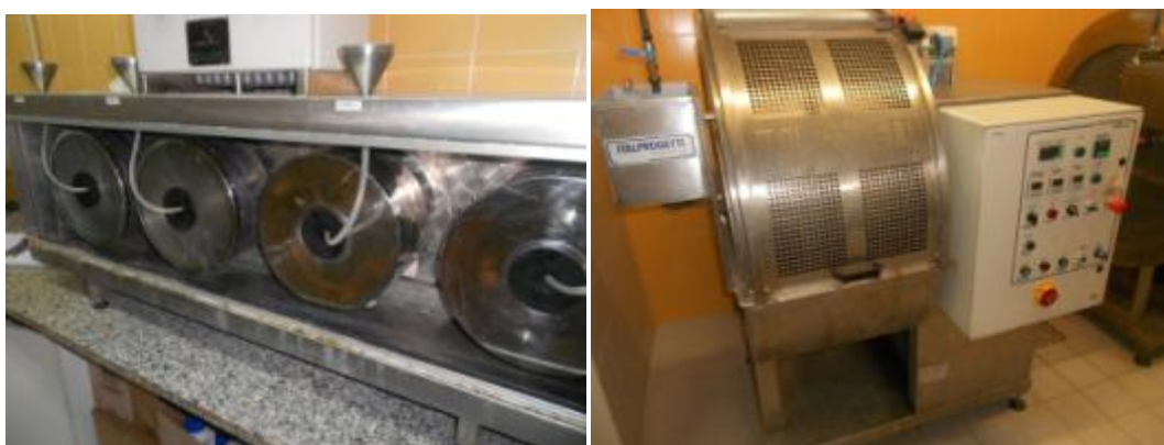
Photo 10: Drums laboratory scale and pilot scale used in this project
