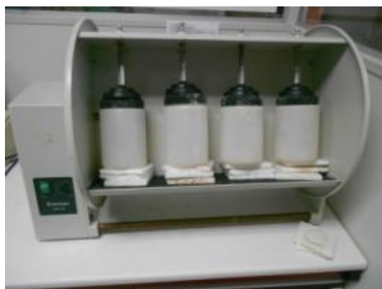
Photo 7: Laboratory Rotary shaker for milling process
