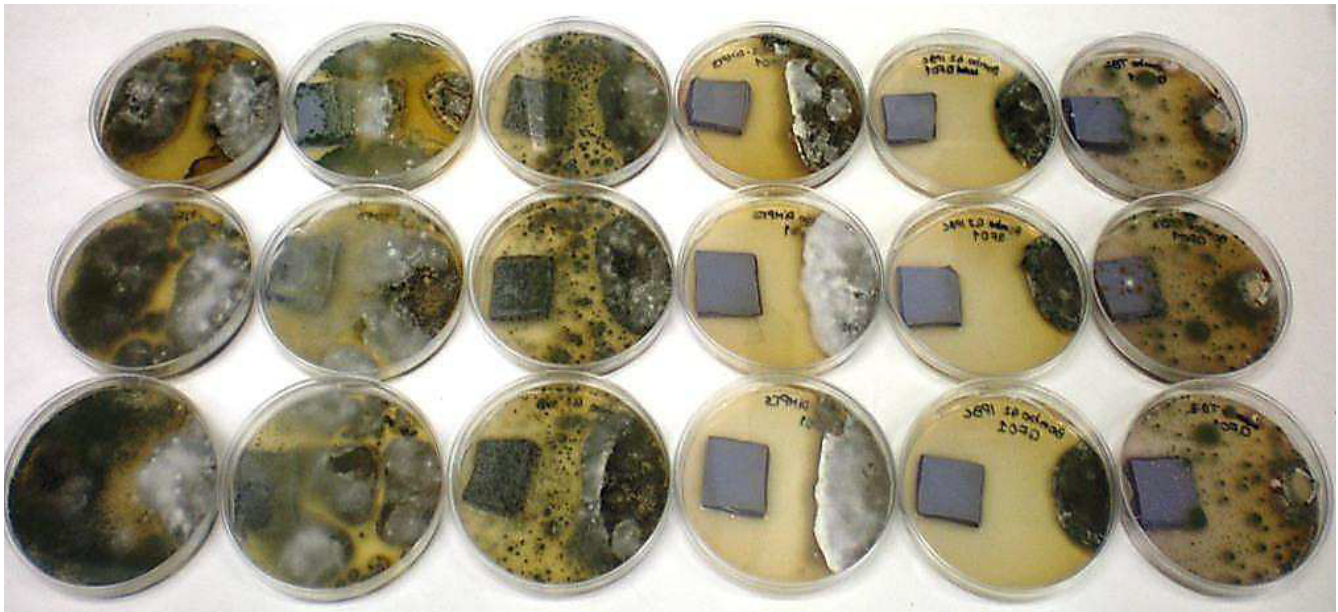
Image 2. Growth of QF01 mould on wet-blue samples after 90 days of testing. From left to right: Control, TCMTB, Mix of phenolics, DIMPTS, IPBC, TBZ.
