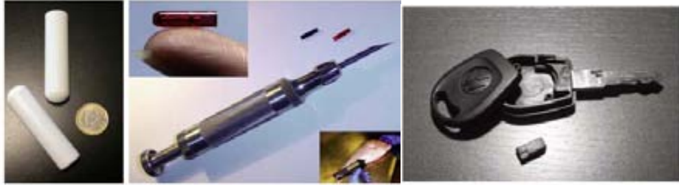
Fig. 2.4 Examples of LF-RFID tags for animal tracking (left) and vehicle immobilizer (right).
