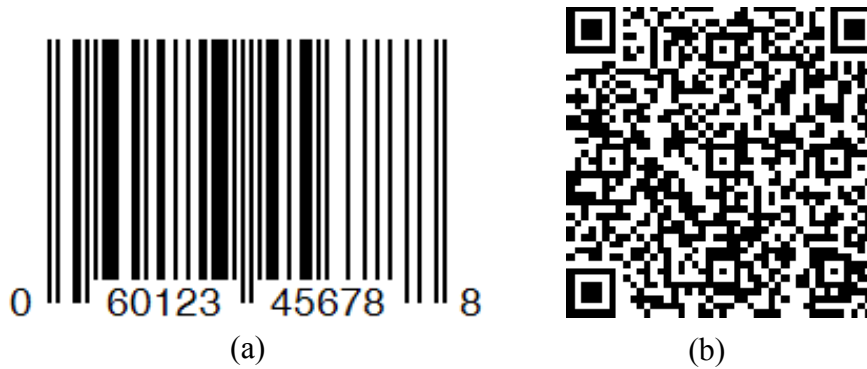
Fig. 2.2 (a) Traditional one-dimensional barcode (UPC code) and (b) two-dimensional barcode (QR code).
