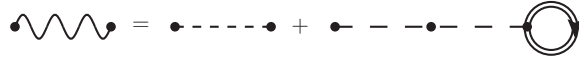
Figure 3.4 – Diagrammatic representation of the effective 2B interaction of Eq. (3.3). This is given by the sum of the original 2B interaction (dashed line) and the 3B interaction (long-dashed line) contracted with a dressed SP propagator, G .
