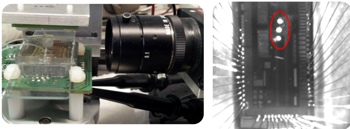
Figure 6.34: On the left side, setup of the system prepared for the optical detection application with the optoelectronic package, the microfluidic chip and the CMOS imaging sensor. Picture on the right side was captured by means of a commercial camera (ALLIED) thanks to a beam splitter placed over a glass substrate. On the right side, photograph of the fabricated CMOS image sensor with 3 active laser spots (red circle) emitted from the VCSELs integrated on the optoelectronic package reported in the previous chapters. These collimated spots are sensed by the image sensor, converted to digital values and processed.
