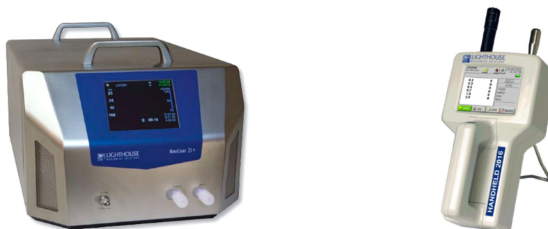
Figure 1.16. Left: Lighthouse NanoCount 25+ portable liquid particle counter. Right: Lighthouse Handheld 2016 airborne particle counter.
