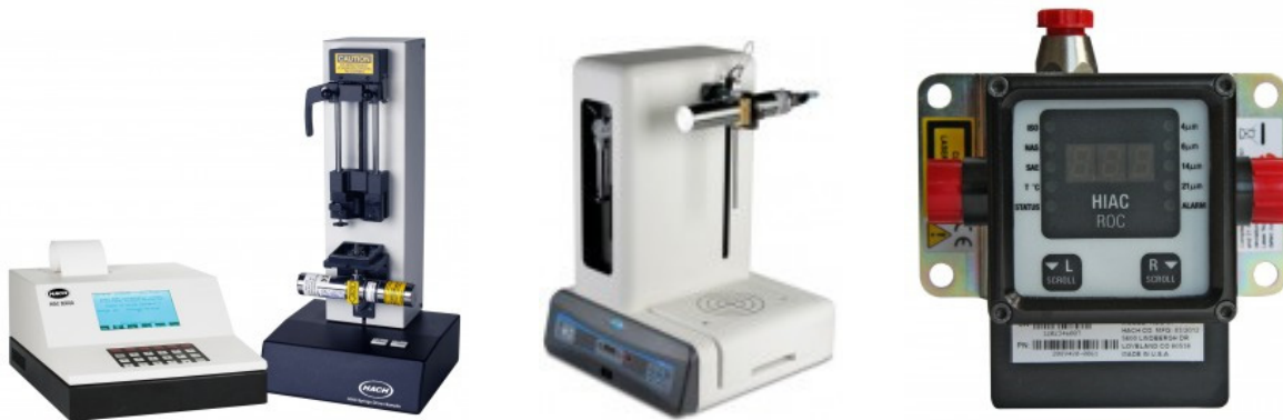
Figure 1.14. HIAC Laboratory particle counters for liquid. Left: HIAC 8012 model ideal for testing dark viscous fluid without dilution (viscosities to 1800 cP) with sample volumes as low as 3 ml. The system includes the 8000A Counter and the Syringe Driven Sampler. Middle: HIAC 9703+ specially designed for pharmaceutical USP <788> quality control and research applications. Device presents dimensions of 343 W, 337 D, 482 H mm and 10.7kg weight. Right: HIAC ROC online liquid particle counters are constructed for industrial harsh environments (high pressure and high temperature applications) offering carefree maintenance.
