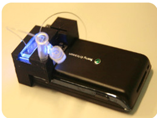
Figure 6.1. Left: Biosensor for fluorescent flow cytometry measurements based on CMOS phone camera as optical detector [5]. Right: Example of application for a CMOS array of pixels combined with a grating coupler [7].
