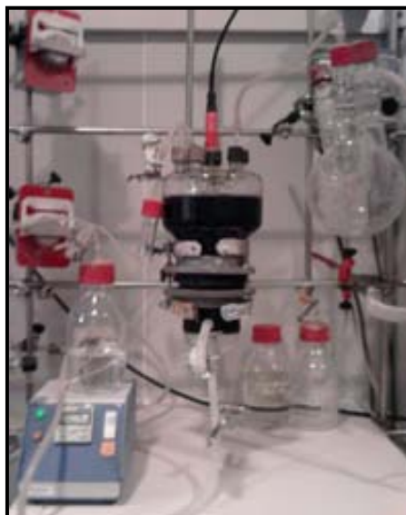
Figure 3.12: Experimental device of the tannery dye decolorization in the reactor
