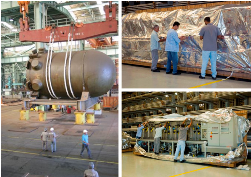
Fig.52: UNA3 imported equipment storage and conservation (Source: www.eletronuclear.gov.br ).
