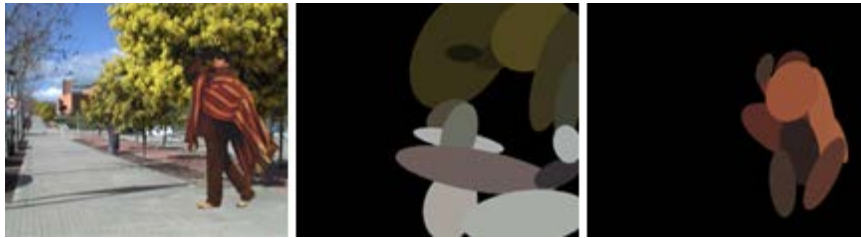
Figure 5.5: Example of foreground and background models. From left to right: input frame under analysis, background model and foreground model. Each ellipse represents one Gaussian of the SCGMM, colored with the mean color that each one is modeling.
