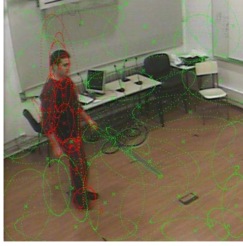
Figure 3.1: Spatial representation of the SCGMM models. Each ellipse is the spatial representation of each Gaussian of the models. Foreground SCGMM in red, background SCGMM in green.
