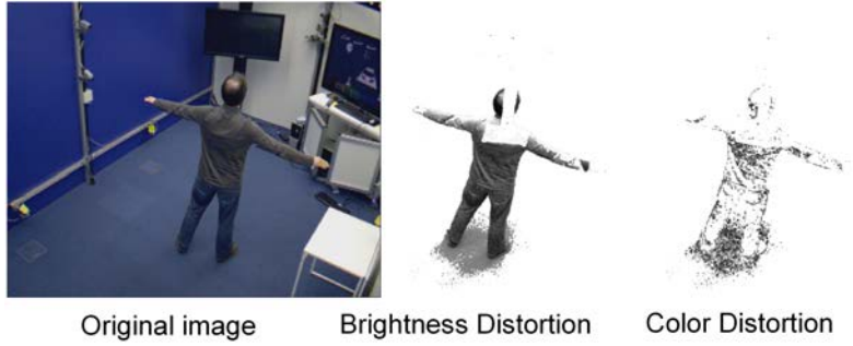
Figure 3.4: Example of brightness distortion BD and color distortion CD domains. Values have been normalized to allow their representation in a gray scale domain. The darker the BD and CD , the smaller their values.
