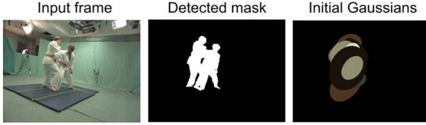
Figure 4.4: Example of GMM initialization. From left to right: Input color frame, corresponding mask of this frame, and the initial foreground SCGMM, where each ellipse corresponds to one Gaussian of the foreground model, filled with the mean color that each one is modeling.
