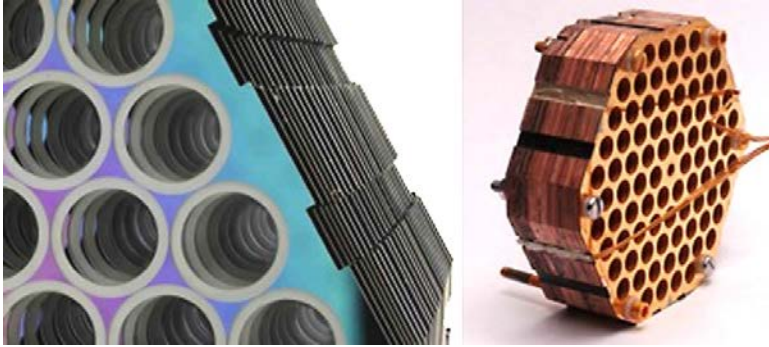
Figure 1.5: (Left) View of silicon platelets before the gold metallization and (Right) view of the fabricated array of horns from [24]
