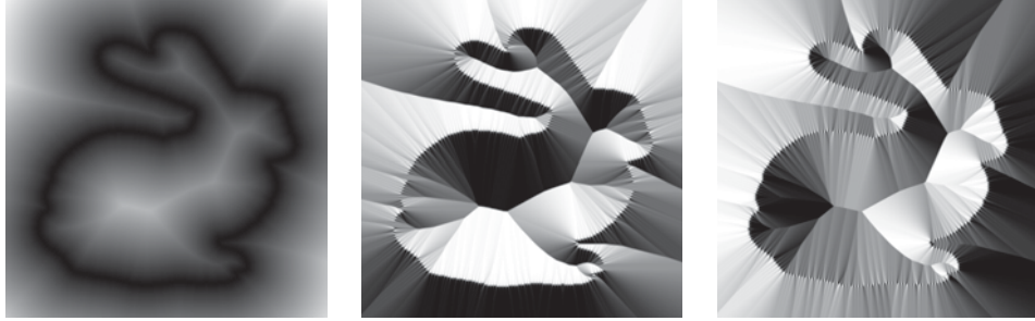
Figure 2.10: Distance field of a 2D bunny point set and its derivatives along two coordinate axes.
