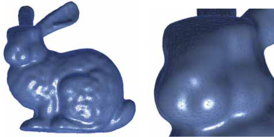
Figure 4.22: ( left ) The efficient 3L-IBS method for fitting a dense set of points. ( right ) Enlargement of a region of the surface.
