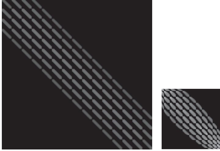
Figure 4.10: The images \log(H) of the regularization matrix H for a cubic control lattice of size N = 15 ; ( left ) when all the control points are considered ( 3375 \times 3375 ); ( right ) when the proposed efficient algorithm is used ( 889 \times 889 )
