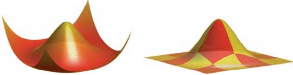
Figure 2.2: Basis functions construct the solution space: ( left ) RBF ; ( right ) IBF.
