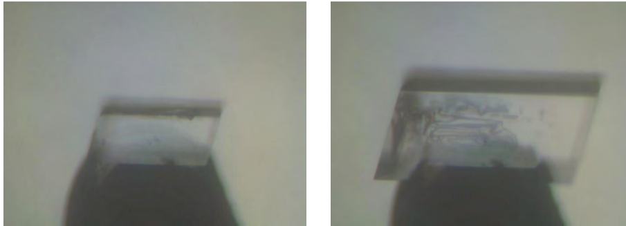
Figure 13. Defects are mainly produced on the back face: dark part within the crystal in the image on the right. T_{\text{growth}} = 297.5 \text{ K} ; \Delta T = 0.8 \text{ K} . Growth time 120 minutes.
