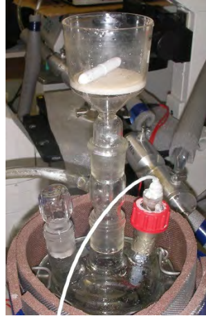
Figure 7. Vacuum filtration inside the reservoir.
