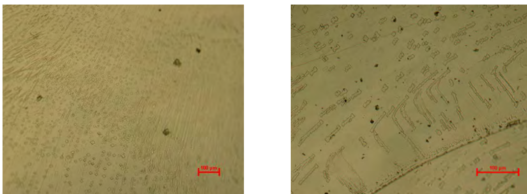
Figure 8. Epitaxial crystallization from an ethanol solution of NaNO 3 onto (104) CaCO 3 . The right figure was taken after rinsing the calcite piece into n-pentane. Samples were in contact with a saturated ethanol solution for 30 minutes before they were dried.
