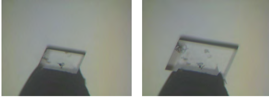
Figure 12. The relative orientation of the faces is not the same as in other images (see figure 13, 14, and figure 10). T_{\text{growth}} = 292.5 \text{ K} ; \Delta T = 0.4 \text{ K} . Growth time 240 minutes.
