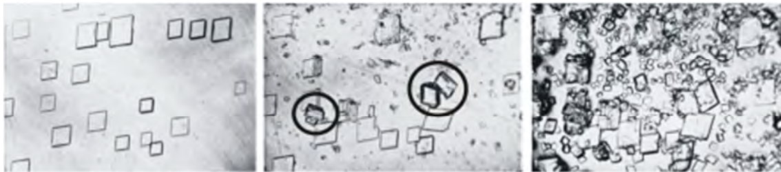
Figure 4. NaNO 3 crystals epitaxially grown on the cleavage {104} rhombohedron of calcite. Déo and Finch (9) - Magnification 60x.
