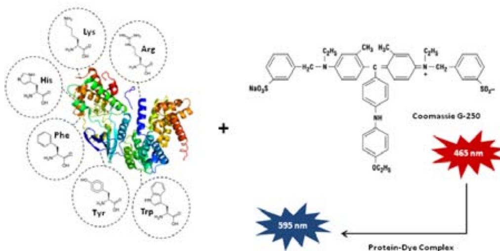
Figure 3.5. Schematic reaction of the Coomassie-based protein assay (Bradford assay).
