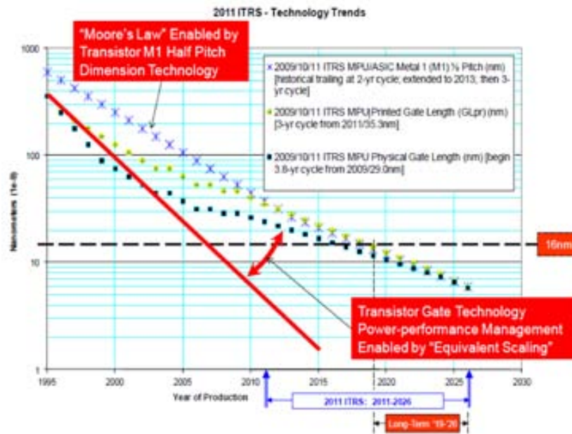
Figure 1.2: MPU (Microprocessor Circuit)/High performance ASIC (Application Specific Integrated Circuit) Half Pitch and Gate Length Trends [1].
