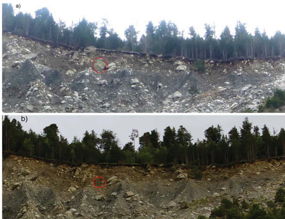
Figure 41: Overview of the steep moraine scarp containing large boulders. The red circle indicates the location of the detachment point of the 2011 rockfall. a) Pre-event photo taken on March 18th 2011, and b) post-event photo taken on May 31st 2011.
