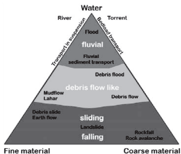
Figure 3: Triangular diagram of torrential and other mass movements, modified after Phillips and Davies (1991), (ONR-24-800, 2007).
