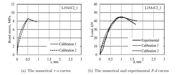
Figure A.6: Calibration curves for specimen L15A1C2-1.
