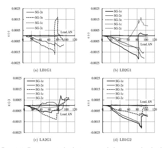
Figure 7.13: Transverse strain distribution on epoxy for beams strengthened with NSM GFRP bars.
