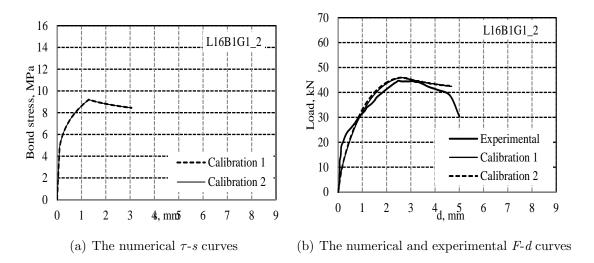
Figure A.13: Calibration curves for specimen L16B1G1-2.
