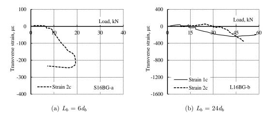
Figure 4.50: Transverse strain distribution on concrete for specimens with GFRP bars bonded with epoxy B.
