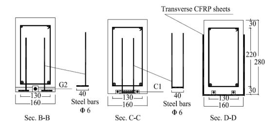
Figure 6.16: Details of the sections of the beams with T and IS.
