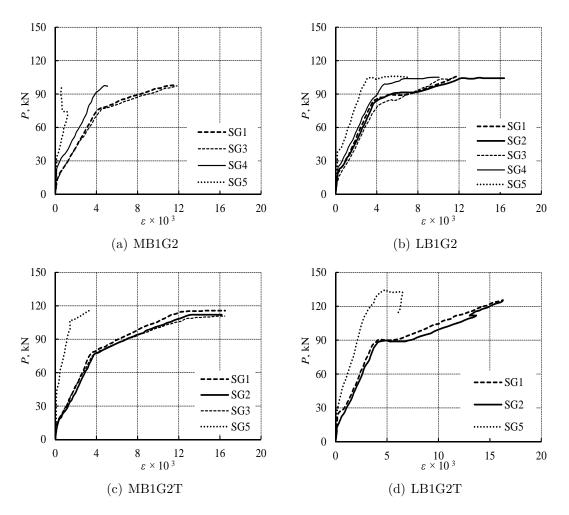
Figure 7.38: Strain in the NSM G2 bars.
