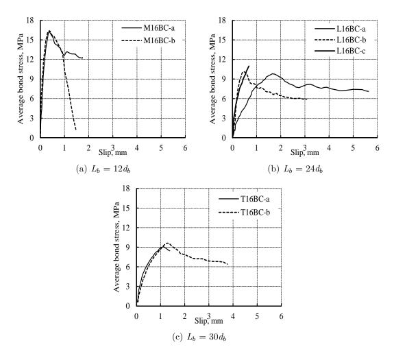
Figure 4.36: Average bond stress slip curves for specimens with CFRP bars bonded with epoxy B.
