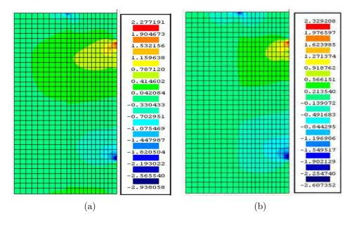
Figure 5.21: FEMIX output (drawmesh) of  $\sigma_{ct}$  along the bonded length ( $F = 0.75F_{max}$  at 1st interface element): (a) L16A1C1-1 and (b) L16A1G1-1.
