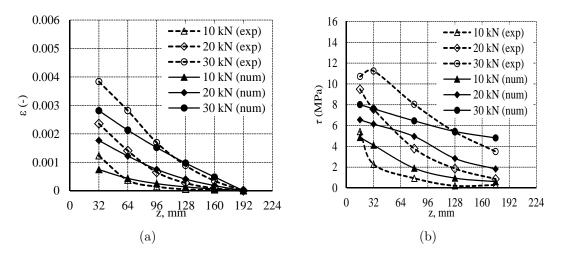
Figure 5.11: Numerical and experimental comparisons: (a) tensile strain and (b) bond shear stress distribution for specimen L12A2C1.
