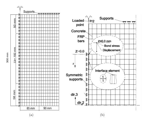
Figure 5.2: Finite element mesh of half of specimen: (a) complete mesh and (b) details of the model.
