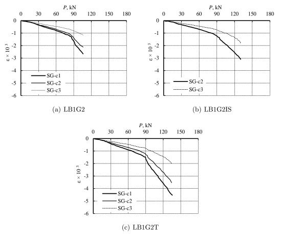
Figure 7.28: Compressive strain in concrete for beams with GFRP bars.
