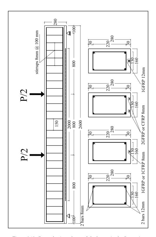
Figure 6.13: Strengthening scheme of the beams in the first series.
