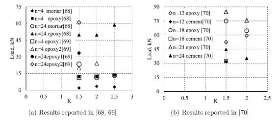
Figure 4.31: Effect of adhesive types on the failure load of tested specimens reported in [[68–70]],  $(K = d/d_b; n = L_b/d_b)$ .
