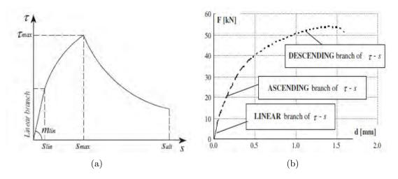
Figure 5.4: (a) local bond stress slip relationship and (b) qualitative correlation between  $\tau - s$  and F-d relationships in a bond test [101].
