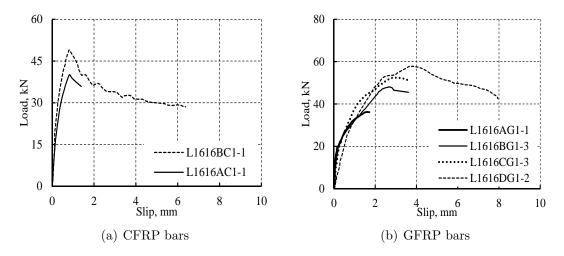
Figure 4.30: Effect of adhesive properties on the behaviour of tested specimens.
