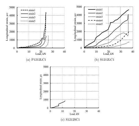
Figure 4.4: Longitudinal strain distributions along the bond length of NSM C1 bars.
