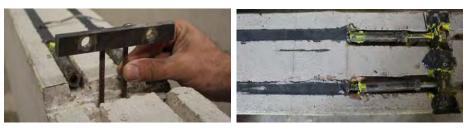
(a) End supporting mechanism for specimen MB2C1ES
