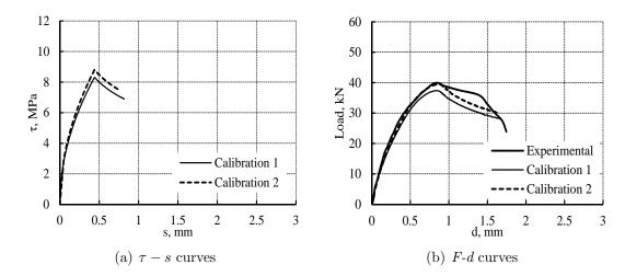
Figure 5.5: Experimental and numerical calibration curves of specimen L16A1C1-1.
