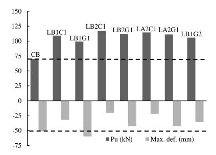
Figure 7.15: Comparison of the load capacity and the corresponding deflection of strengthened beams.
