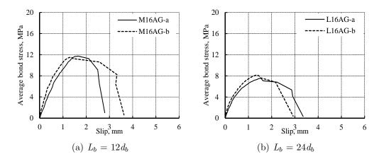
Figure 4.44: Average bond stress slip curves for specimens with GFRP bars bonded with epoxy A.
