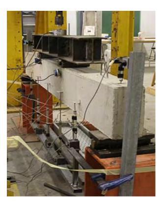
Figure 6.9: Arrangement of the vertical transducers and inclinometers.
