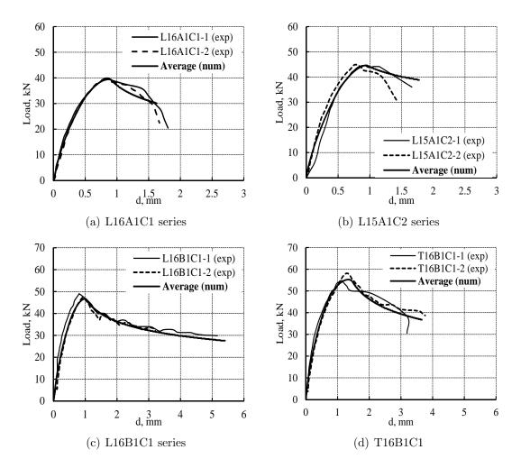
Figure 5.6: Experimental and numerical F-d curves of specimens with CFRP bars (concrete 1).
