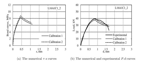
Figure A.1: Calibration curves for specimen L16A1C1-2.
