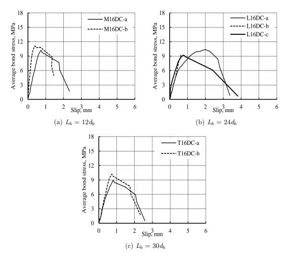
Figure 4.37: Average bond stress slip curves for specimens with CFRP bars bonded with epoxy D.
