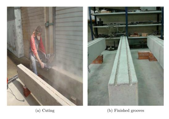
Figure 6.4: Formation of the grooves in the tension side of beams.
