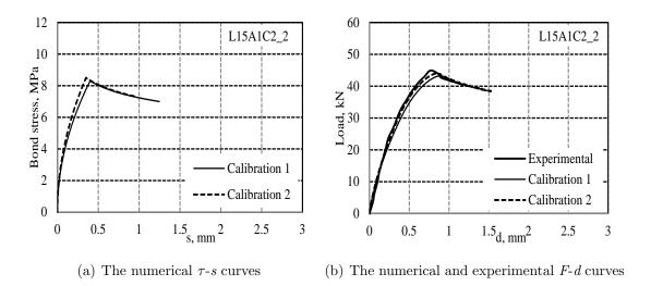
Figure A.7: Calibration curves for specimen L15A1C2-2.
