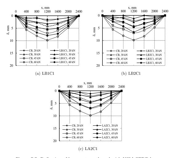
Figure 7.7: Deflection of beams strengthened with NSM CFRP bars.
