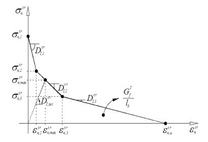
Figure 5.3: Trilinear stress strain diagram to simulate the fracture mode I crack propagation ( $\sigma_{n,2}^{cr} = \alpha_1 \sigma_{n,1}^{cr}$ ,  $\sigma_{n,3}^{cr} = \alpha_2 \sigma_{n,1}^{cr}$ ,  $\varepsilon_{n,2}^{cr} = \xi_1 \ \varepsilon_{n,u}^{cr}$ ,  $\varepsilon_{n,3}^{cr} = \xi_2 \ \varepsilon_{n,u}^{cr}$ ).
