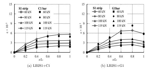
Figure 7.24: Strain distribution along half of the FRP reinforcement.
