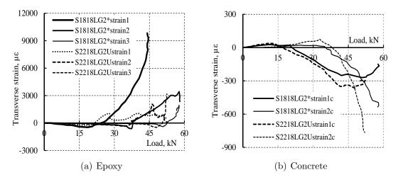
Figure 4.9: Effect of the inside concrete part confinement on the transverse strain.
