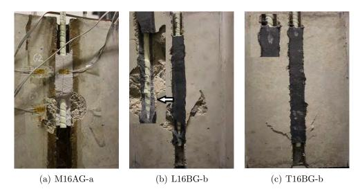
Figure 4.43: Failure mode of specimens with GPRP bars.
