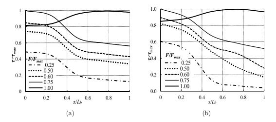
Figure 5.16: Longitudinal bond stress distributions along the bond length for specimens of NSM FRP bars: (a) L16A1C1-1 and (b) L16A1G1-1.
