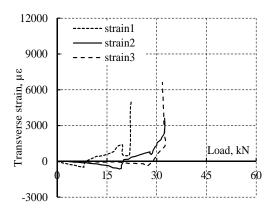
Figure 4.23: Transverse strain distribution for specimen L1616AG1I.
