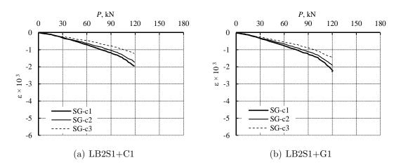
Figure 7.27: Compressive strain in concrete for beams with combined FRPR.
