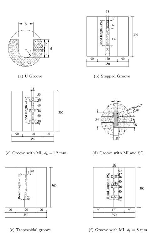
Figure 3.7: NSM configurations (dimensions in mm).
