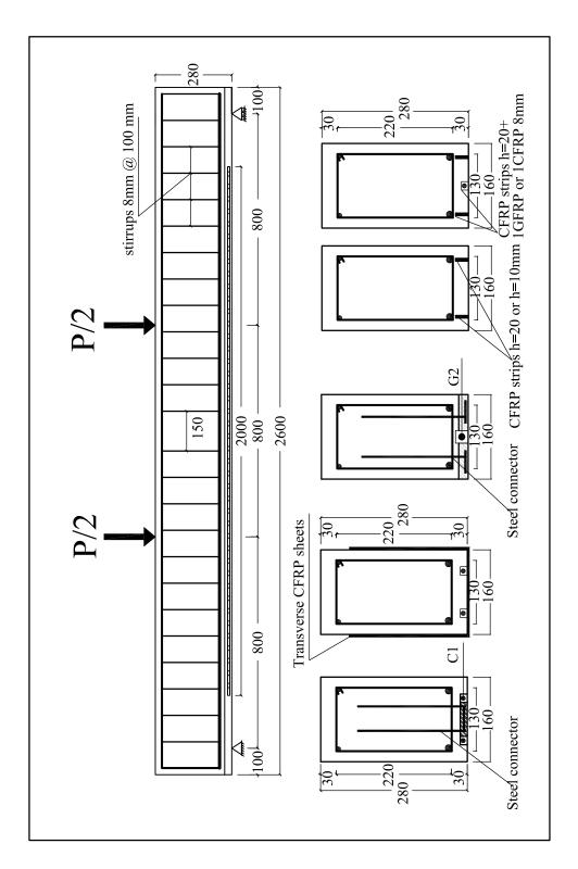
Figure 6.14: Strengthening scheme of the beams in the second series.
