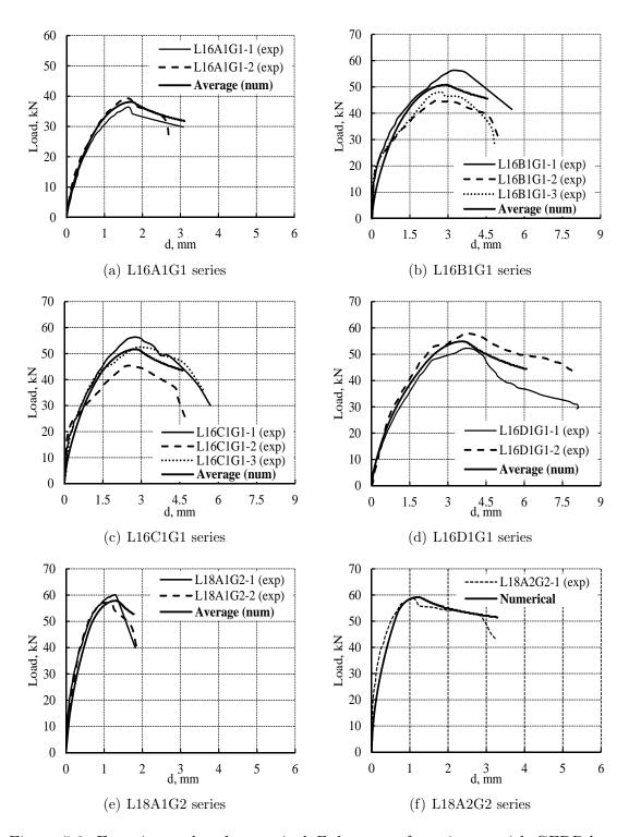
Figure 5.9: Experimental and numerical F-d curves of specimens with GFRP bars.
