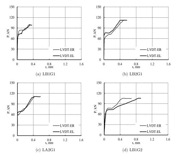
Figure 7.10: Free end slip curves of beams strengthened with GFRP bars.
