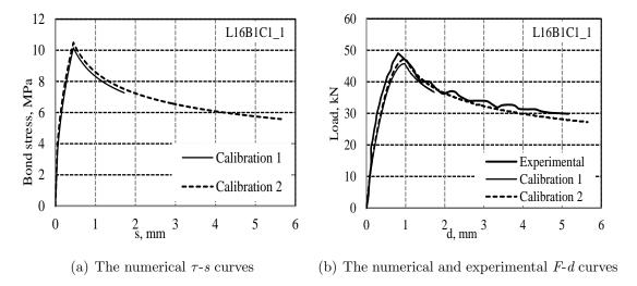
Figure A.2: Calibration curves for specimen L16B1C1-1.
