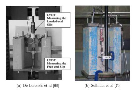
Figure 3.1: Pullout tests arrangements.
