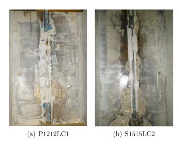
Figure 4.1: Failure modes of specimens with CFRP bars.
