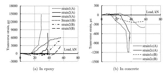
Figure 4.32: Transverse strain distribution for specimens L1616AG1 and L1616BG1.
