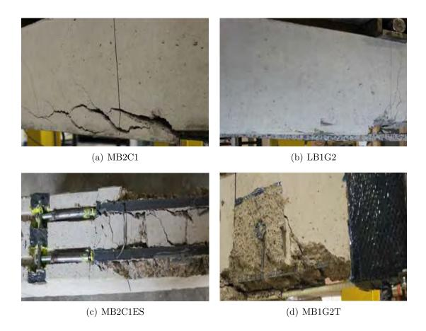
Figure 7.33: Modes of failure of the tested RC beams.
