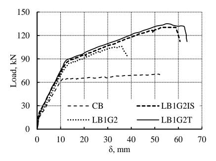
Figure 7.21: Effect of mechanical interlocking with shear connectors and transverse wrapping on the load deflection curve of the strengthened beams with GFRP bars.
