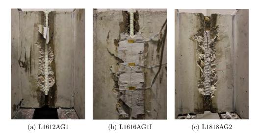
Figure 4.16: Failure mode of specimens with NSM GFRP bars bonded with adhesive type A.
