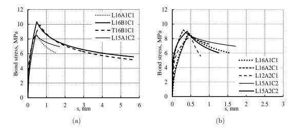
Figure 5.8: Comparisons of the  $\tau - s$  curves of specimens with CFRP bars: a) influence of the bar size and adhesive properties; b) influence of the concrete strength and groove size.
