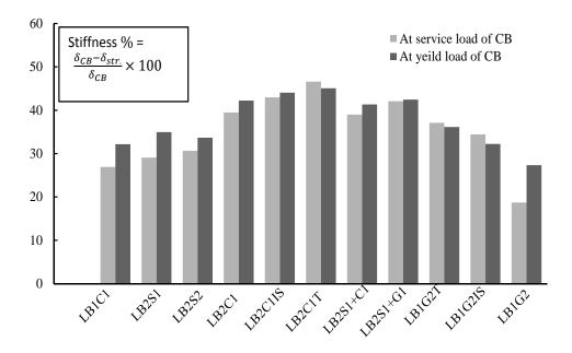
Figure 7.22: Comparison of stiffness of strengthened beams at service load and at yielding load of the CB.
