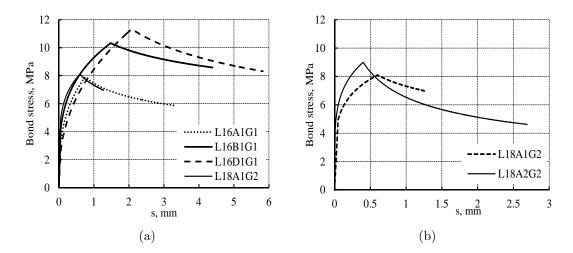
Figure 5.10: Comparisons of the  $\tau-s$  curves of specimens with GFRP bars: (a) influence of the bar size and adhesive properties and (b) influence of the concrete strength.
