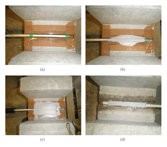
Figure 3.4: Bonding of NSM bars.
