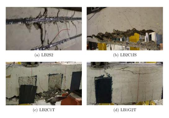
Figure 7.17: Modes failure of the tested RC beams.
