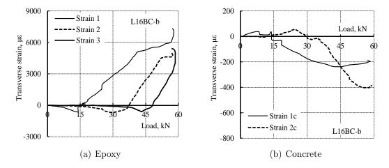
Figure 4.40: Transverse strain distribution for specimens with CFRP bars bonded with epoxy B (L16BC-b).
