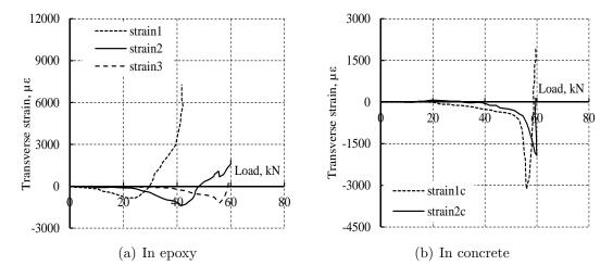
Figure 4.24: Transverse strain distribution for specimen L1818AG2.
