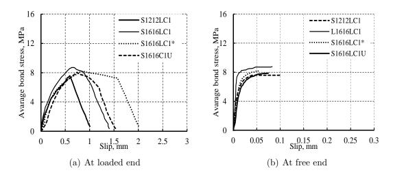
Figure 4.3: Effect of the inside concrete part confinement and groove geometry on the behaviour of specimens with NSM C1 bars.
