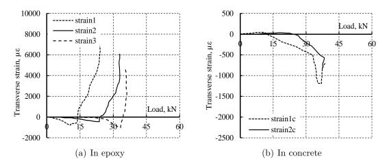
Figure 4.21: Transverse strain distribution for specimen L1620AG1T.
