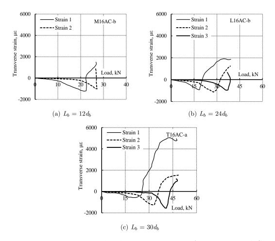
Figure 4.38: Transverse strain distribution on epoxy paste for specimens with CFRP bars bonded with epoxy A.
