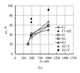
Figure 7.47: Effect of NSM reinforcement on the load efficiency of the strengthened RC beams: (a) at yield load and (b) at ultimate load.
