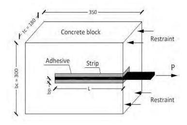
Figure 2.8: Test specimen configuration and setup [76].
