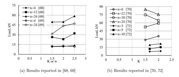
Figure 4.29: Effect of groove dimensions and bond length on the capacity of specimens reported in [68–70, 72],  $(K = d/d_b; w = \text{groove width}; n = L_b/d_b; L_b = \text{bond length}).$
