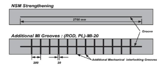
Figure 2.12: Plan view of the NSM strengthening with mechanical interlocking grooves [90].
