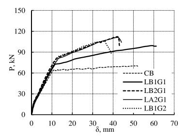
Figure 7.8: Load deflection curve of beams strengthened with NSM GFRP bars.
