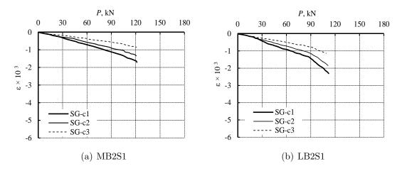
Figure 7.40: Compressive strain in concrete for beams with NSM CFRP strips.
