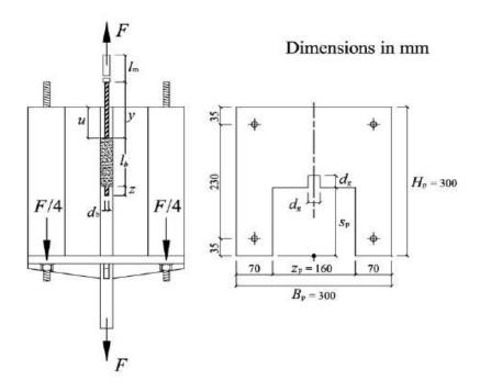
Figure 2.5: Test specimen configuration of the modified pullout test [68].
