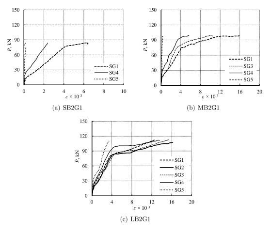
Figure 7.37: Strain in the NSM G1 bars.
