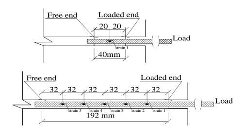
(a) Longitudinal strain gauges on FRP bars
