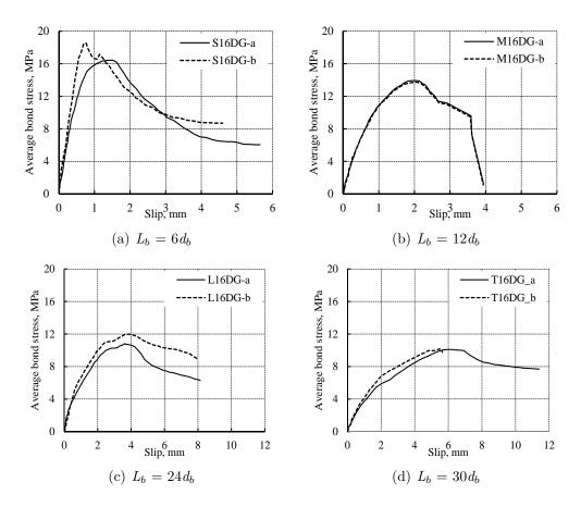
Figure 4.46: Average bond stress slip curves for specimens with GFRP bars bonded with epoxy D.
