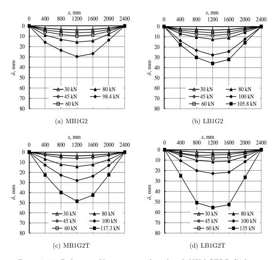
Figure 7.46: Defection of beams strengthened with NSM GFRP G2 bars.
