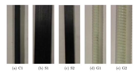
Figure 6.12: Surface treatment of the FRP reinforcement used in the flexural test.
