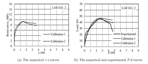
Figure A.16: Calibration curves for specimen L16C1G1-2.
