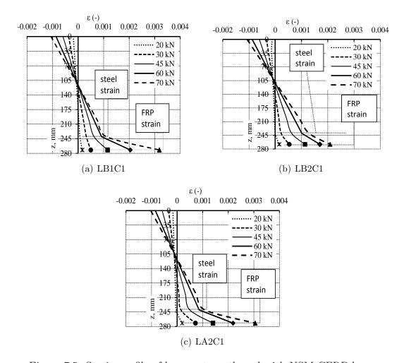
Figure 7.5: Strain profile of beams strengthened with NSM CFRP bars.
