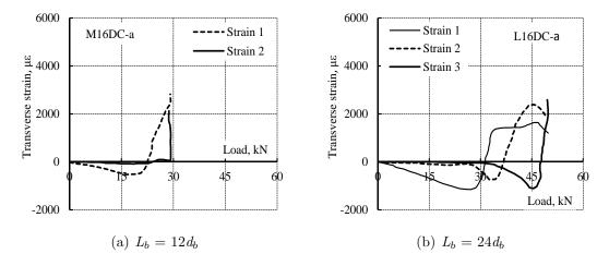
Figure 4.41: Transverse strain distribution on epoxy for specimens with CFRP bars bonded with epoxy D.
