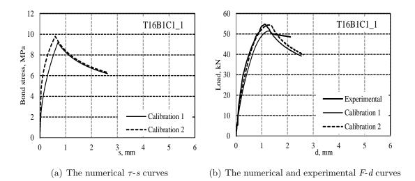
Figure A.4: Calibration curves for specimen T16B1C1-1.
