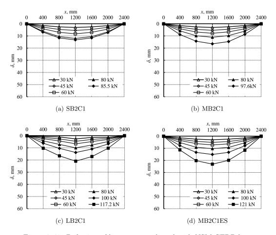
Figure 7.43: Defection of beams strengthened with NSM CFRP bars.
