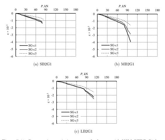
Figure 7.41: Compressive strain in concrete for beams with NSM GFRP G1 bars.
