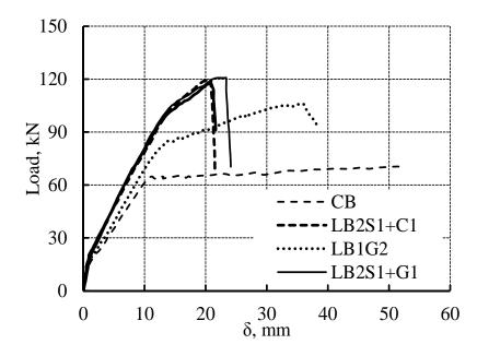
Figure 7.19: Effect of NSM material and arrangement on the load deflection curve of the strengthened beams.
