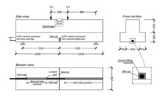
Figure 2.9: Test specimen configuration and setup of beam pullout test [77].
