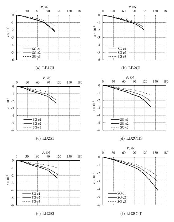
Figure 7.26: Compressive strain in concrete for beams with CFRP reinforcement.
