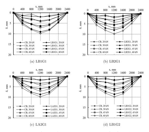
Figure 7.14: Deflection of beams strengthened with NSM GFRP bars.
