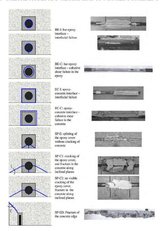
Figure 2.16: Bond failure modes of NSM systems observed in bond tests [38].
