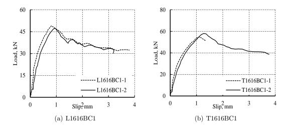
Figure 4.13: Load slip curves of specimens with NSM CFRP bars bonded with epoxy type B.
