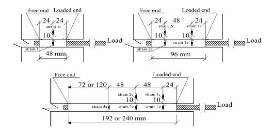
(b) Transverse strain gauges on concrete (c) and epoxy (e) surfaces
