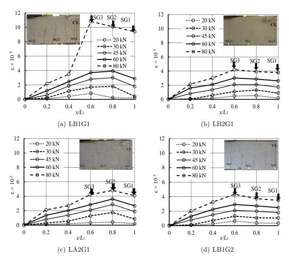
Figure 7.11: Strain distribution along half of the NSM GFRP bars.
