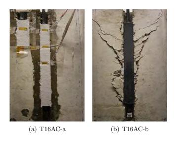
Figure 4.34: Failure mode of specimens with CFRP bars.
