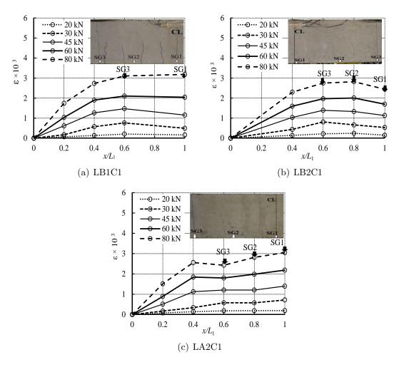
Figure 7.4: Strain distribution along half of the NSM CFRP bars.
