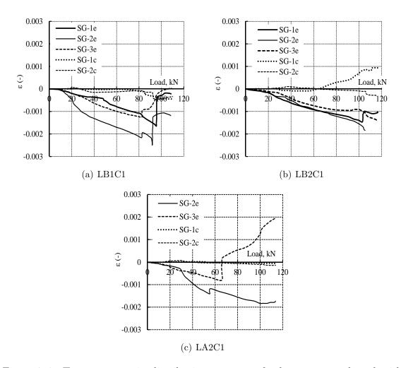
Figure 7.6: Transverse strain distribution on epoxy for beams strengthened with NSM CFRP bars.
