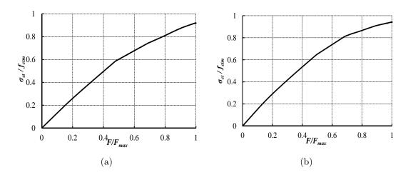
Figure 5.19: Theoretical distribution of normalized tensile stresses in the concrete: (a) L16A1C1-1 and (b) L16A1G1-1.
