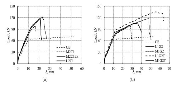
Figure 7.34: Effect of end anchorage of the NSM bars and transverse wrapping on the load deflection curve of the strengthened beams: (a) C1 bars and (b) G2 bars.
