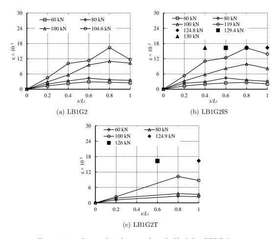
Figure 7.25: Strain distribution along half of the GFRP bars.
