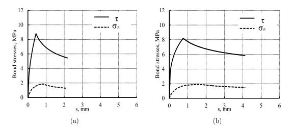
Figure 5.18: Distribution of bond shear stress in the first interface element and tensile stress in the first concrete element at the loaded end: (a) L16A1C1-1 and (b) L16A1G1-1.
