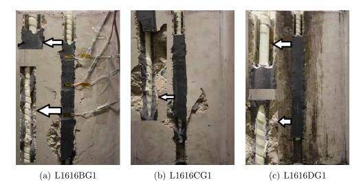
Figure 4.17: Failure mode of specimens with NSM GFRP bars bonded with adhesive types B, C and D.
