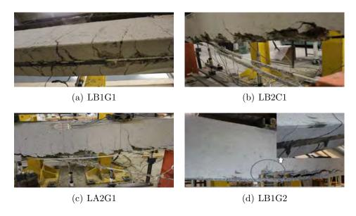
Figure 7.9: Failure modes of beams strengthened with NSM GFRP bars.
