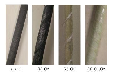
Figure 3.2: Surface treatment of the FRP bars.
