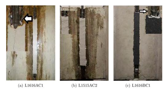
Figure 4.11: Failure modes of specimens with NSM CFRP bars.
