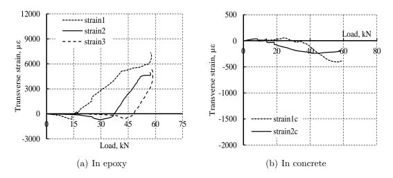
Figure 4.25: Transverse strain distribution for specimen L1616BG1.
