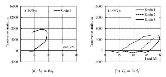
Figure 4.49: Transverse strain distribution on epoxy for specimens with GFRP bars bonded with epoxy B.
