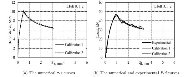
Figure A.3: Calibration curves for specimen L16B1C1-2.
