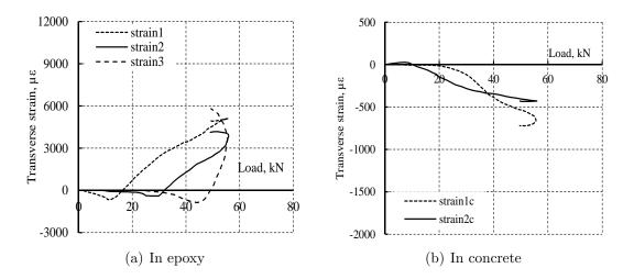
Figure 4.26: Transverse strain distribution for specimen L1616CG1.
