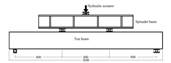
Figure 6.7: Flexural test setup.
