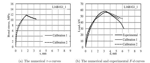
Figure A.12: Calibration curves for specimen L16B1G1-1.
