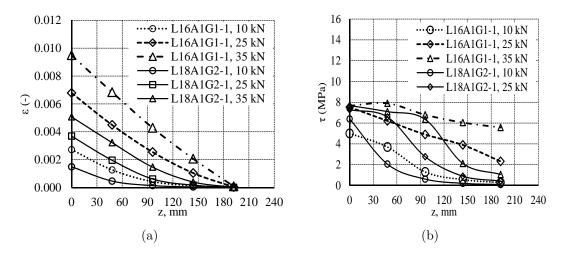
Figure 5.13: Effect of bar size on the: (a) strain distribution and (b) bond stress distribution.
