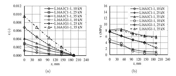
Figure 5.12: Effect of FRP type on the: (a) strain distribution and (b) bond stress distribution.
