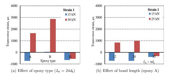
Figure 4.54: Effect of epoxy type and bond length on the transverse strain of NSM CFRP bars.
