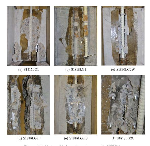
Figure 4.5: Modes of failure of specimens with GFRP bars.
