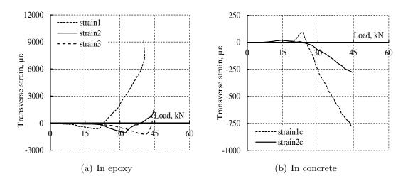
Figure 4.15: Transverse strain distribution for specimen L1515AC2.
