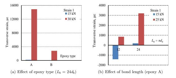
Figure 4.55: Effect of epoxy type and bond length on the transverse strain of NSM GFRP bars.
