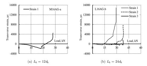
Figure 4.47: Transverse strain distribution on epoxy for specimens with GFRP bars bonded with epoxy A.
