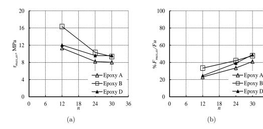
Figure 4.52: Effect of epoxy type and bond length for specimens with CFRP bars on: (a)  $\tau_{max,av}$  and (b)  $\%F_{max,av}$   $/F_u$ ;  $(n = L_b/d_b)$ .
