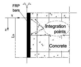
Figure 5.17: Scheme for the calculation of tensile stress in the concrete in the transverse plane.
