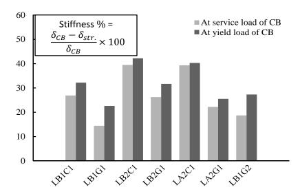
Figure 7.16: Comparison of stiffness of strengthened beams at service load and at yielding load of the CB.
