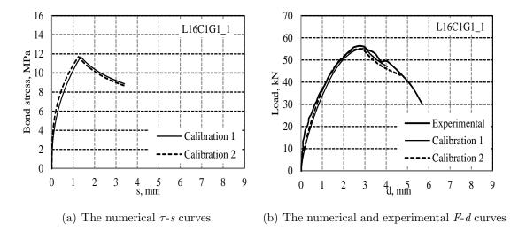
Figure A.15: Calibration curves for specimen L16C1G1-1.
