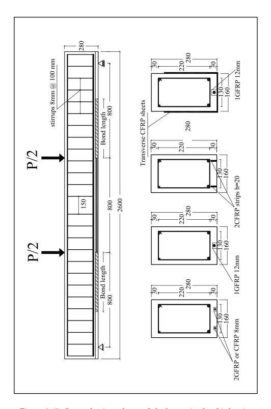
Figure 6.17: Strengthening scheme of the beams in the third series.
