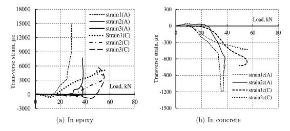
Figure 4.33: Transverse strain distribution for specimens L1616AG1 and L1616CG1.
