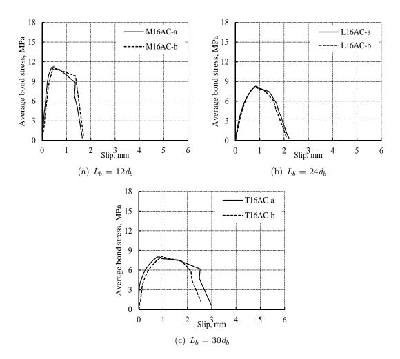
Figure 4.35: Average bond stress slip curves for specimens with CFRP bars bonded with epoxy A.
