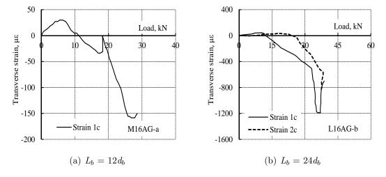
Figure 4.48: Transverse strain distribution on concrete for specimens with GFRP bars bonded with epoxy A.
