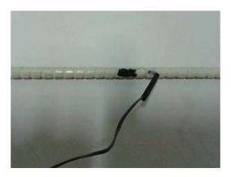
Figure 6.11: Strain gauges on the NSM bars.
