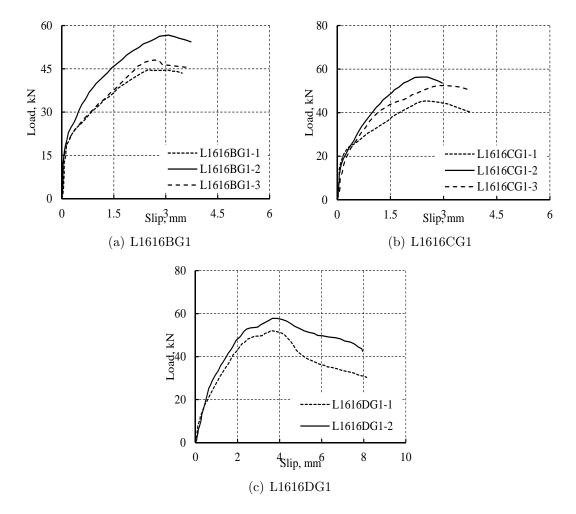
Figure 4.19: Load slip curves of specimens with NSM GFRP bars bonded using epoxy types B,C and D.
