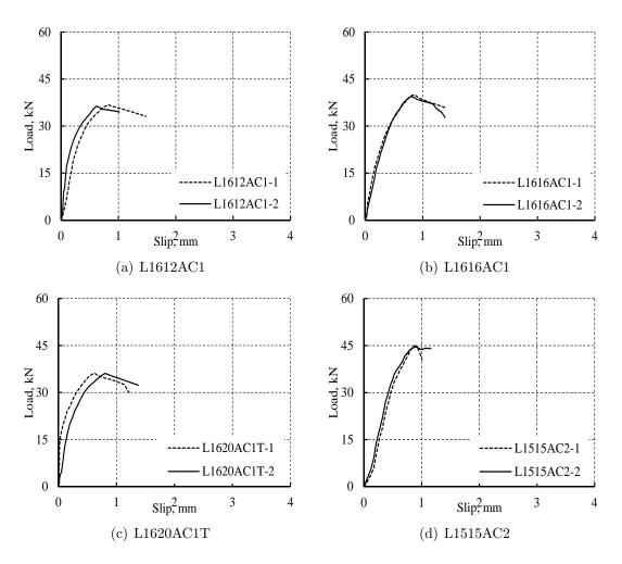
Figure 4.12: Load slip curves of specimens with NSM CFRP bars bonded with epoxy type A.
