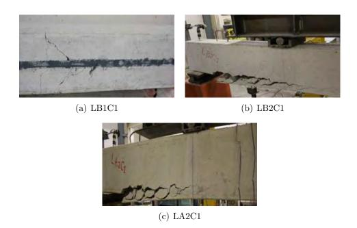
Figure 7.2: Failure modes of beams strengthened with NSM CFRP bars.
