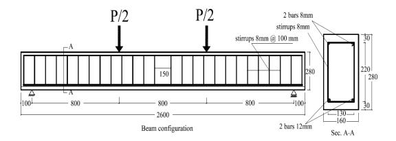
Figure 6.1: Dimensions and reinforcement details of the RC beam.
