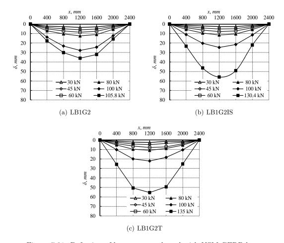
Figure 7.31: Defection of beams strengthened with NSM GFRP bars.
