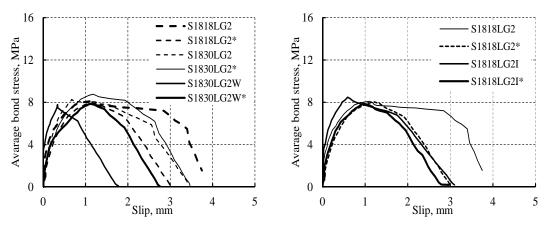
(a) Specimens with different groove dimensions (b) Effect of confinement on specimens had MI
