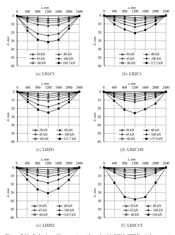
Figure 7.30: Defection of beams strengthened with NSM CFRP reinforcement.
