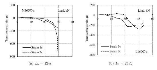
Figure 4.42: Transverse strain distribution on concrete for specimens with CFRP bars bonded with epoxy D.
