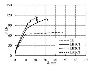
Figure 7.1: Load deflection curve of beams strengthened with NSM CFRP bars.
