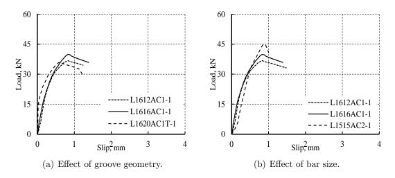
Figure 4.27: Effect of groove dimensions, geometry and bar size on behaviour of specimens with NSM CFRP bars.
