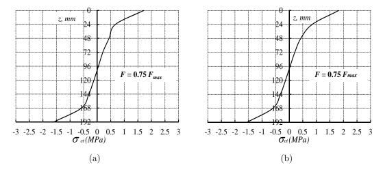
Figure 5.20: Distribution of  $\sigma_{ct}$  along the bonded length ( $F = 0.75F_{max}$  at 1st interface element): (a) L16A1C1-1 and (b) L16A1G1-1.
