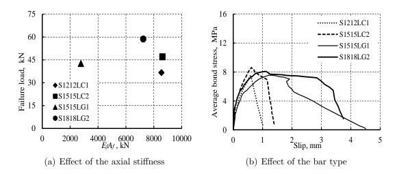
Figure 4.10: Behaviour of specimen with different FRP bars.
