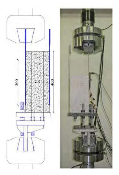
Figure 2.7: Test specimen configuration and setup of the single shear test [71].
