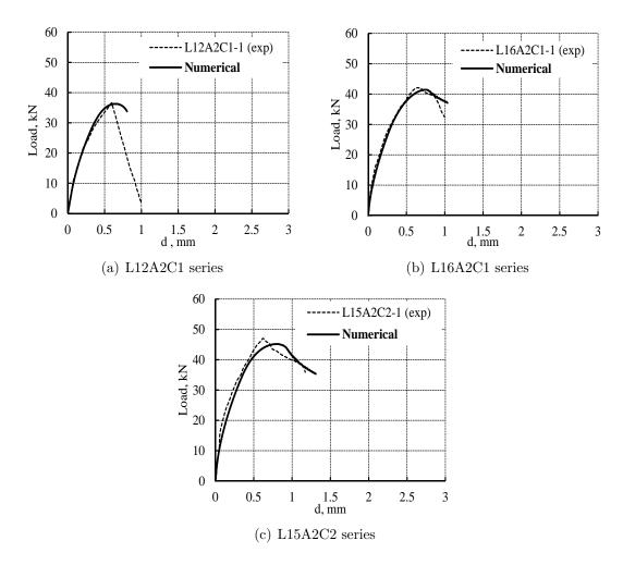
Figure 5.7: Experimental and numerical F-d curves of specimens with CFRP bars (concrete 2).
