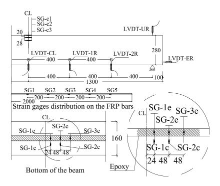
Figure 6.8: Sketch of the tested beams instrumentation.
