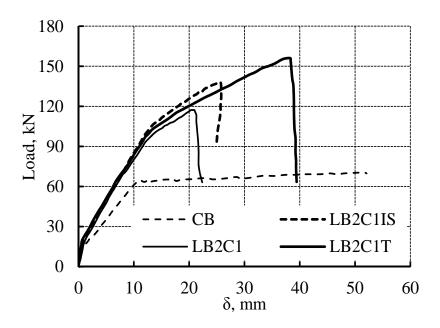
Figure 7.20: Effect of mechanical interlocking with shear connectors and transverse wrapping on the load deflection curve of the strengthened beams with CFRP bars.
