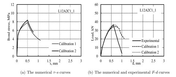
Figure A.10: Calibration curves for specimen L12A2C1-1.
