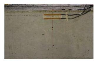
Figure 6.10: Arrangement of the concrete strain gauges in the mid-span top section.
