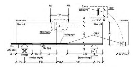
Figure 2.10: Beam pullout test setup [78].
