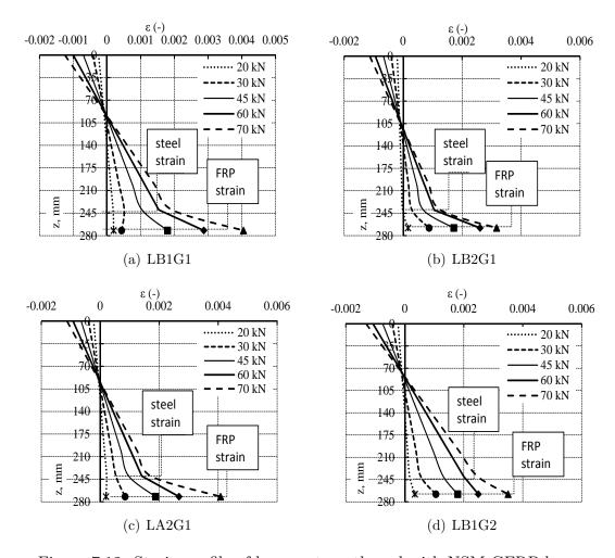
Figure 7.12: Strain profile of beams strengthened with NSM GFRP bars.
