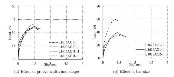
Figure 4.28: Effect of groove width, shape and FRP bar size on behaviour of specimens with NSM GFRP bars.
