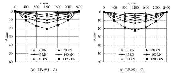
Figure 7.29: Defection of beams strengthened with combined NSM FRP reinforcement.
