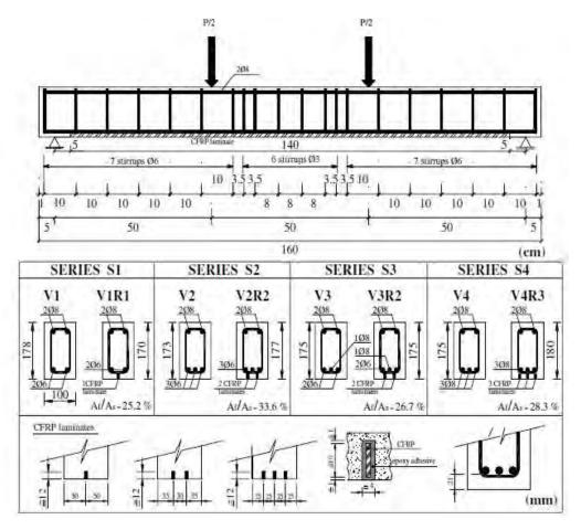
Figure 2.14: Details of the tested beams [21].
