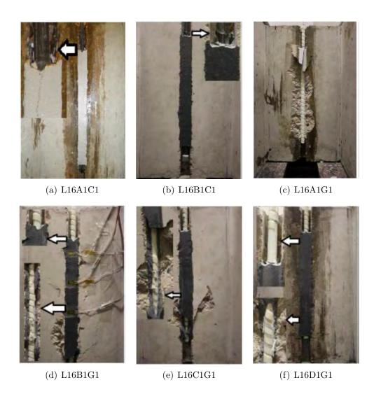
Figure 5.1: Failure mode of the tested specimens.
