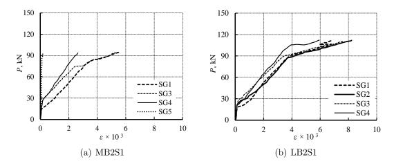
Figure 7.36: Strain in the NSM CFRP strips.
