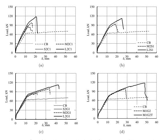
Figure 7.32: Effect of bond length on the load deflection curve of the strengthened beams: (a) C1 bars, (b) S1 strips, (c) G1 bars and (d) G2 bars.
