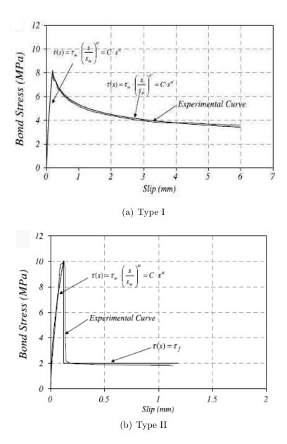
Figure 2.11: Typical bond slip curves of NSM FRP reinforcement [15].
