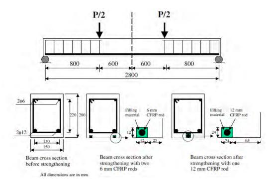
Figure 2.13: Details and setup of the tested beams [27].
