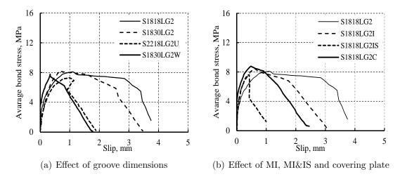
Figure 4.6: Average bond stress slip curves of NSM GFRP bars.
