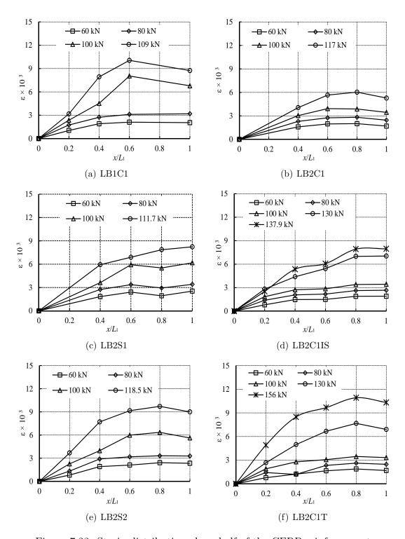
Figure 7.23: Strain distribution along half of the CFRP reinforcement.
