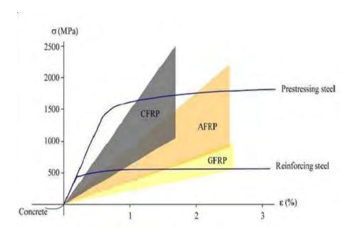
Figure 2.2: A comparison of the tensile properties of FRP and steel bars [44].
