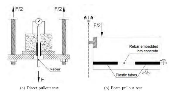
Figure 2.4: Test setup for direct and beam pullout tests [42].
