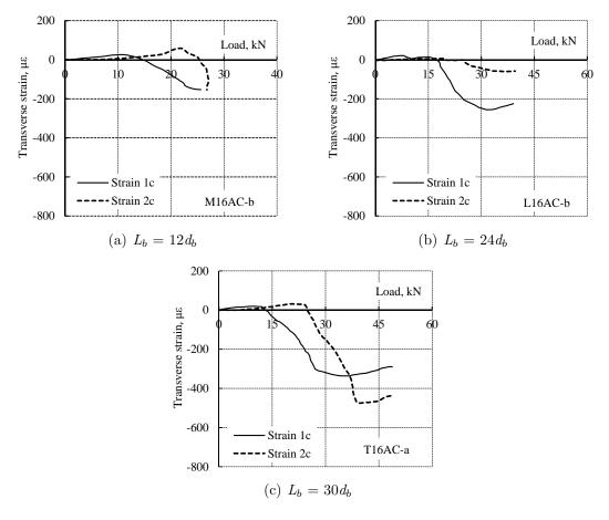
Figure 4.39: Transverse strain distribution on concrete for specimens with CFRP bars bonded with epoxy A.
