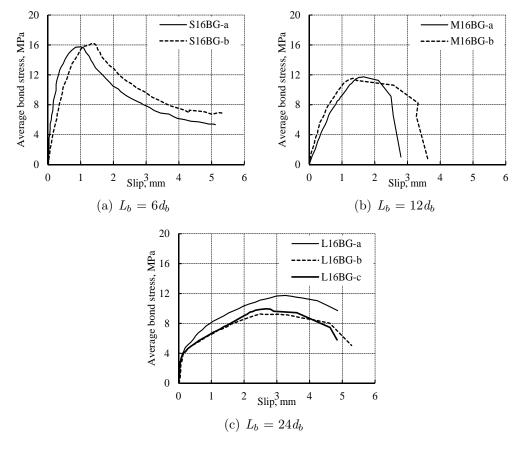
Figure 4.45: Average bond stress slip curves for specimens with GFRP bars bonded with epoxy  ${\bf B}$ .
