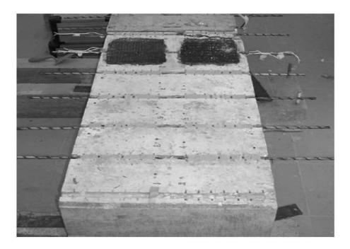
Figure 2.6: Test specimen configuration of the modified pullout test [69].
