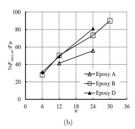
Figure 4.53: Effect of epoxy type and bond length for specimens with GFRP bars on: (a)  $\tau_{max,av}$  and (b)  $\%F_{max,av}$   $/F_u$ ;  $(n = L_b/d_b)$ .
