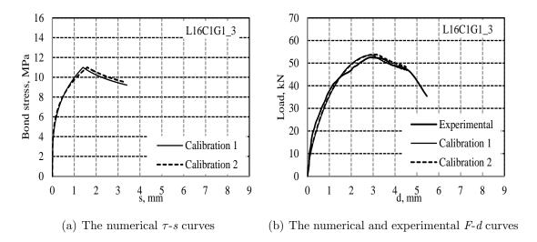
Figure A.17: Calibration curves for specimen L16C1G1-3.
