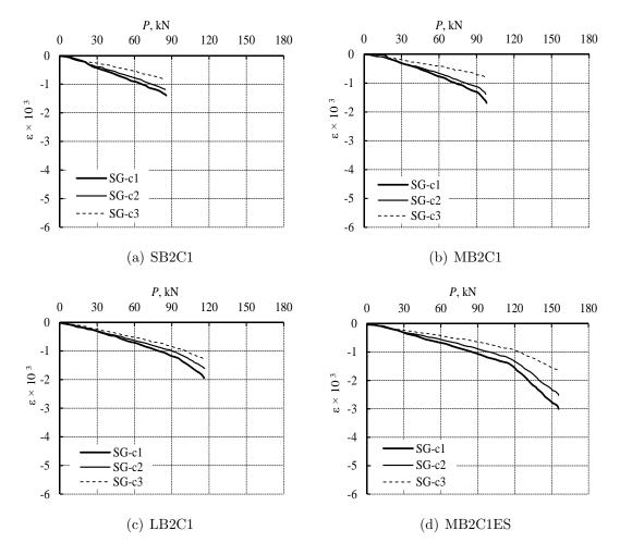
Figure 7.39: Compressive strain in concrete for beams with NSM CFRP bars.
