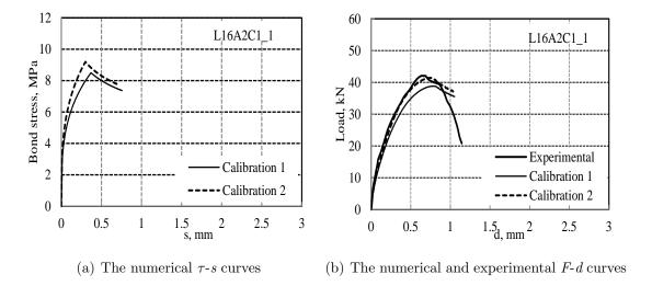
Figure A.8: Calibration curves for specimen L16A2C1-1.
