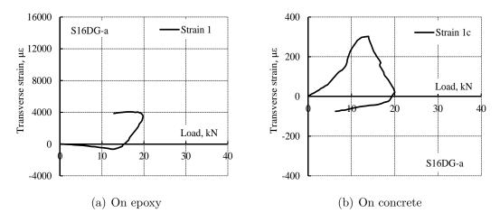
Figure 4.51: Transverse strain distribution for specimens with GFRP bars bonded with epoxy D (S16DG-a).
