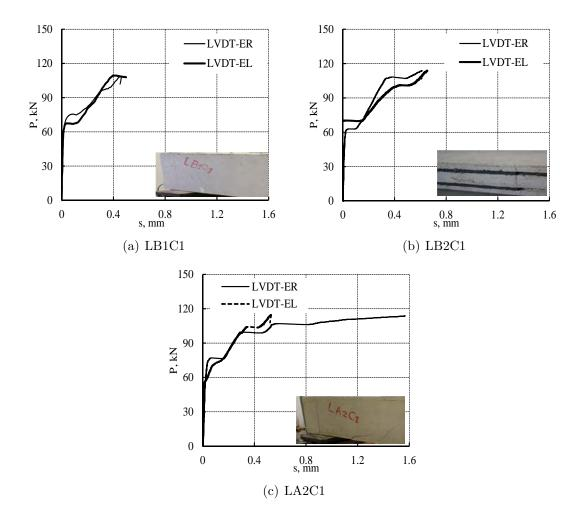
Figure 7.3: Free end slip curves of beams strengthened with CFRP bars.
