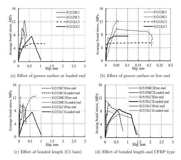
Figure 4.2: Average bond stress slip curves of NSM CFRP bars.
