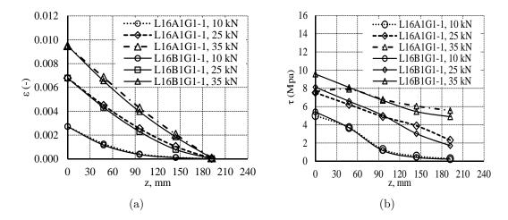
Figure 5.14: Effect of adhesive type on the: (a) strain distribution and (b) bond stress distribution.
