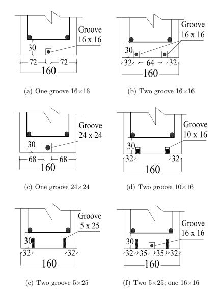
Figure 6.5: Full details and locations of the grooves for the strengthened beams.
