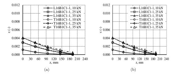
Figure 5.15: Effect of bond length on the: (a) strain distribution and (b) bond stress distribution.
