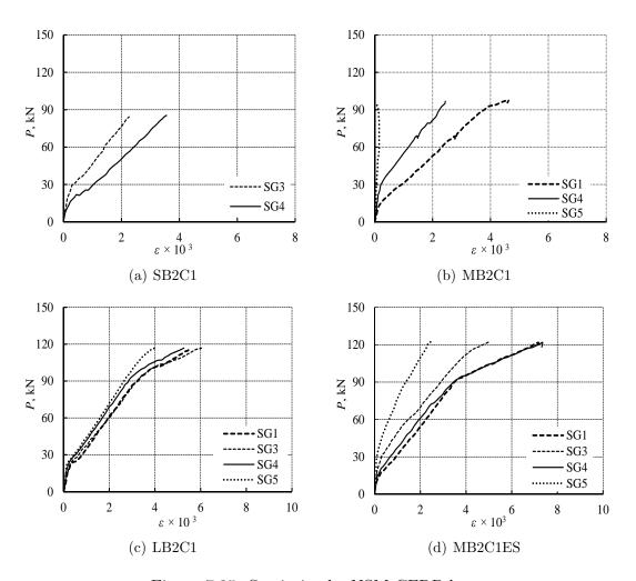
Figure 7.35: Strain in the NSM CFRP bars.
