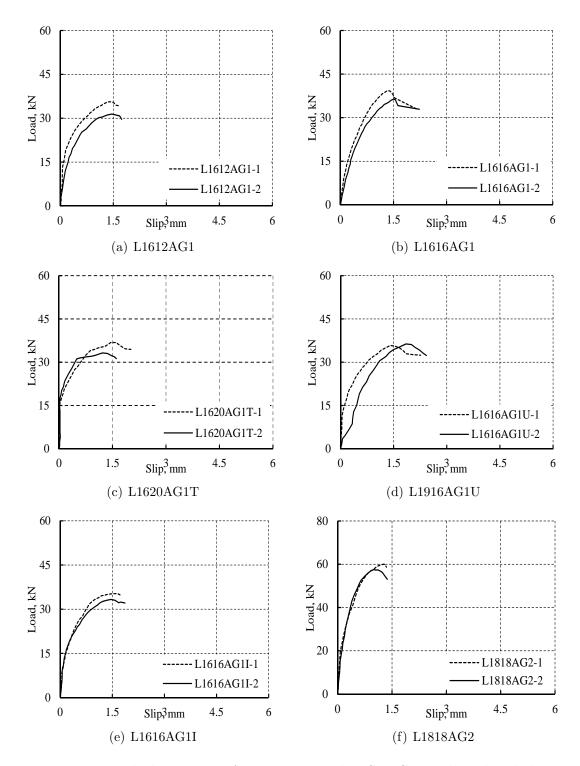
Figure 4.18: Load slip curves of specimens with NSM GFRP bars bonded using epoxy type A.
