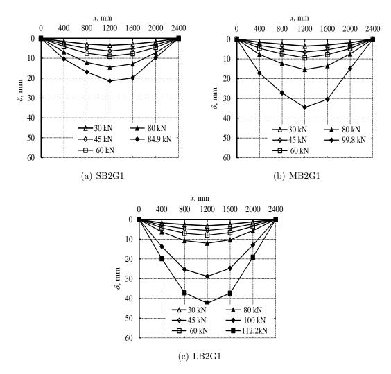
Figure 7.45: Defection of beams strengthened with NSM GFRP G1 bars.
