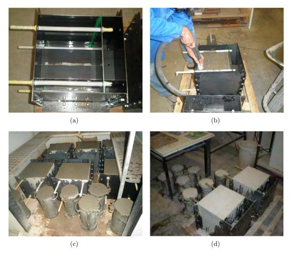
Figure 3.3: Mould preparation and casting.
