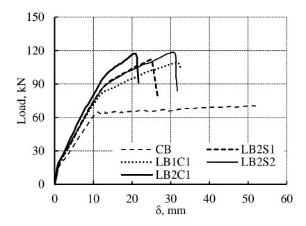
Figure 7.18: Effect of NSM shape, dimensions and area on the load deflection curve of the strengthened beams.
