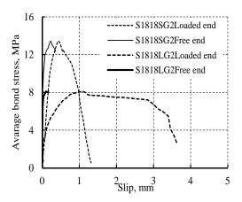
Figure 4.8: Effect of bond length on the behaviour of specimens with NSM G2 bars.
