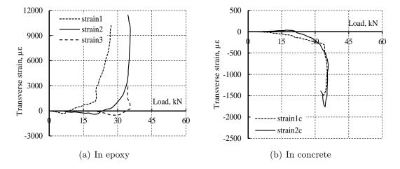
Figure 4.22: Transverse strain distribution for specimen L1916AG1U.
