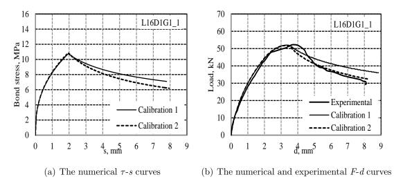
Figure A.18: Calibration curves for specimen L16D1G1-1.
