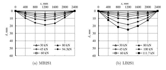
Figure 7.44: Defection of beams strengthened with NSM CFRP strips.
