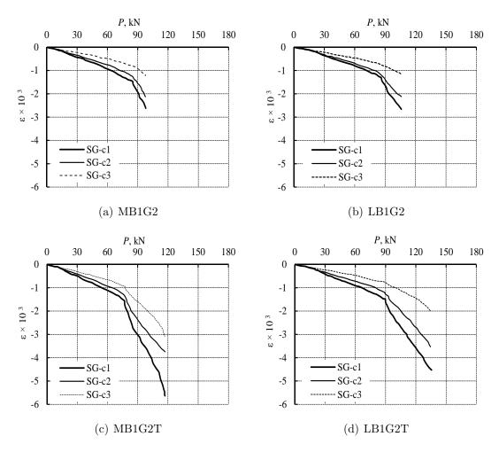
Figure 7.42: Compressive strain in concrete for beams with NSM GFRP G2 bars.
