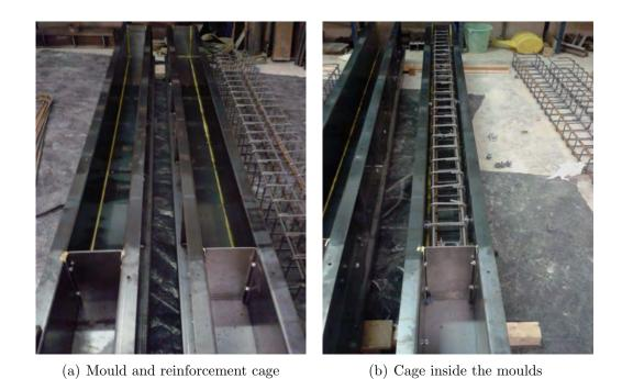
Figure 6.2: Appearance of the mould and reinforcement.
